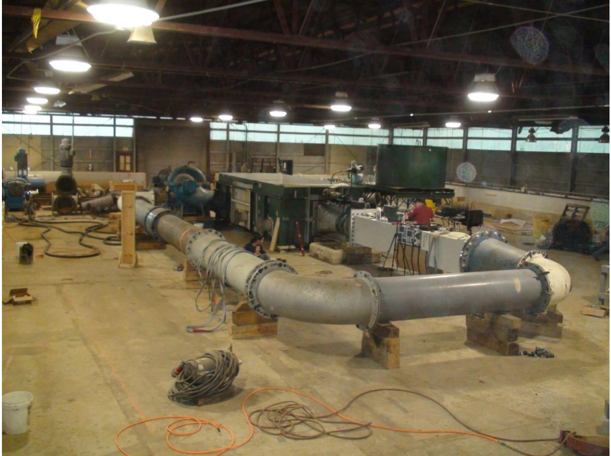
Figure 7 Sub Scale Turbine Test Loop at Alden Labs
