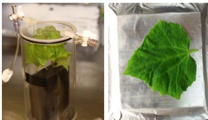
Figure 9. (L) Photographs of a plant labeling chamber with a cucumber plant inside. (R) A radiolabeled leaf on top of the phoswich detector being imaged by the hybrid imager.
