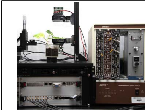
Figure 3. The hybrid imager consists of a gamma detector, a phoswich detector, NIM electronics, and an ADC system.
