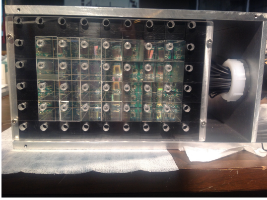
Figure 1: A prototype of the (g-2) -calorimeter, tested at SLAC. This test-box consisted of a 4 \times 7 PbF 2 crystal array with each crystal coupled to a Hamamatsu SiPM.
