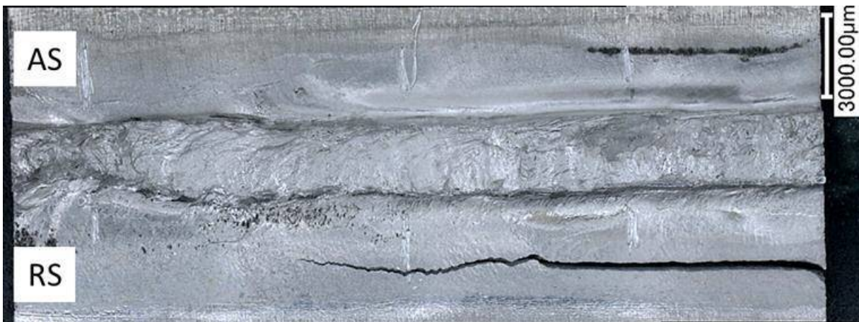
Figure 18. Plan view of fatigue fracture for a lap-shear specimen of 1.5 mm AA6022-T4 joined to AM60B die-cast magnesium. AS = advancing side, RS = retreating side of weld pin motion.
