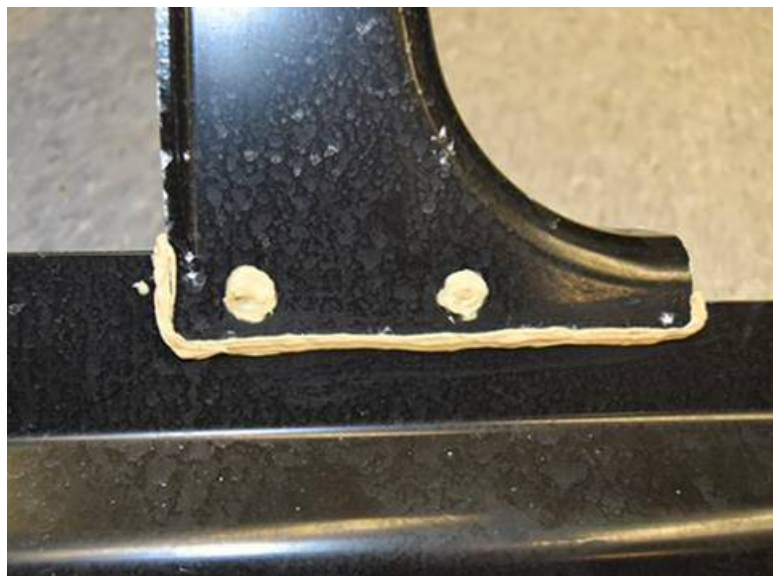
Figure 58. Example of ‘sealed’ lower-rail joint for steel-upper corrosion test structure with coverage of rivet caps and lap areas. Internal adhesive placement is not visible.
