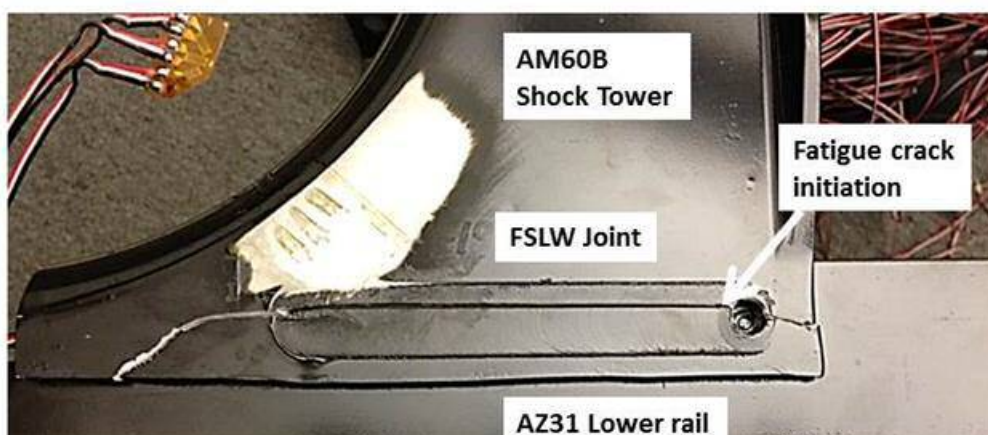
Figure 20. Fatigue crack initiation at tool extraction point and traverse across FSLW joint in Phase II demonstration structure.
