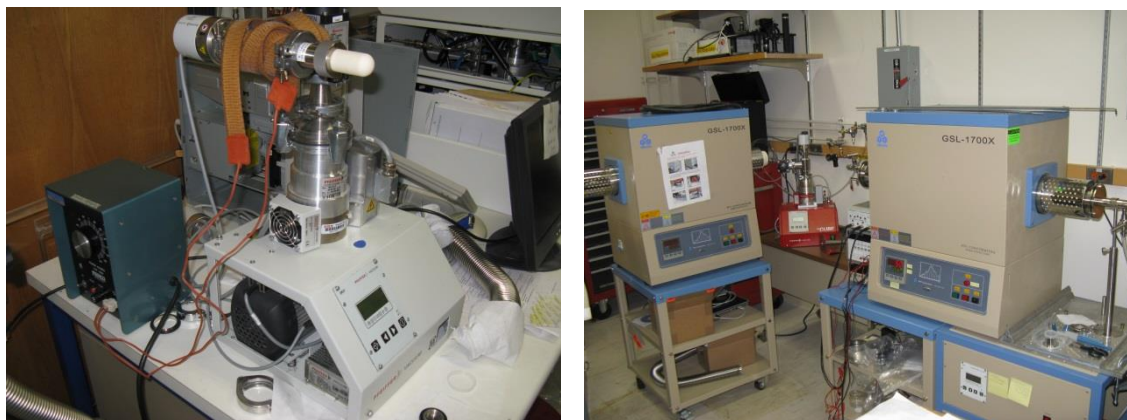
Figure 2. Pfeiffer Turbo Pump and Two MTI 1700 °C Vacuum Oven
