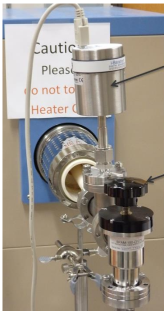
Figure 8. Pressure measurement and turbo pump setup.
