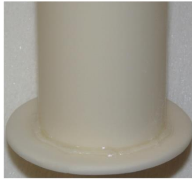
After firing, can see that some of sealant material flowed
