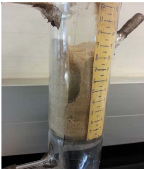
Figure 2.4. Channeling observed in the cold fluidization units of biomass and coal/biomass mixtures.
