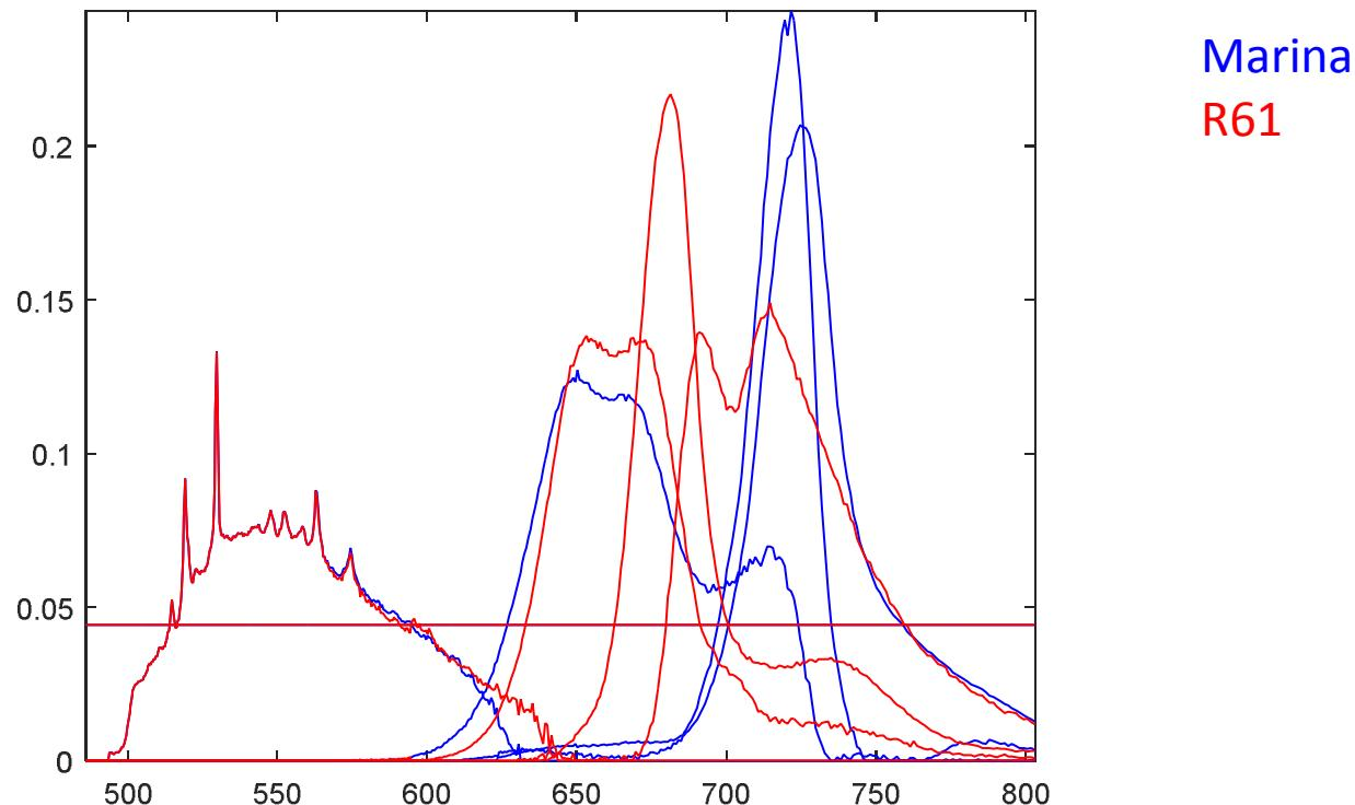
Both of these have a significant residual at the point of the spectrum of the highest intensity, most likely from the non-linear detector response. These were taken at OD 1.0 and the laser power may have been a bit too high. Spectral deconvolution is challenging because there's not enough variation in the data set. Would be improved if we had cells under two conditions that promoted phycobilisome /chl ratio changes.
