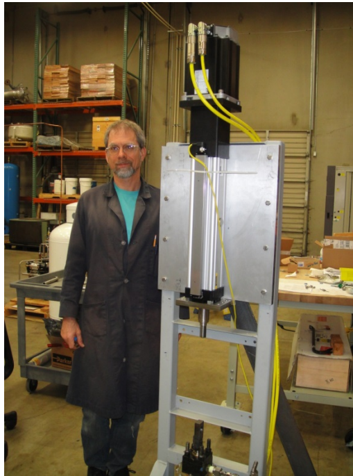
Figure 10. A picture of the programmable, reversing ball-screw linear actuator for the magnetic regenerator drive subsystem. This actuator is on the test stand in this picture. It is mounted on top of the cold box lid during AMRR operation. One of the two yellow cables is the electrical power cable and the other one is the controls cable.
