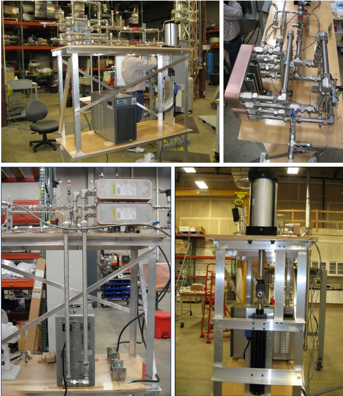
Figure 13. Heat Transfer Fluid (HTF) subsystem components and the AMRR drive actuator (bottom right) with coupling to HTF positive displacement pump. The chiller coupling to HTF circuit (bottom left picture) allows controllable T_H temperature.
