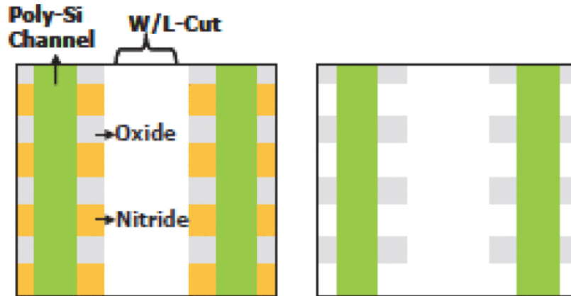
(a) After 'W/L cut' dry etch (b) Wet removal of nitride
