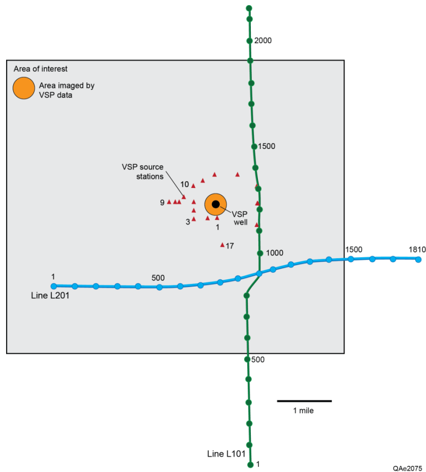
Figure 4.46. Location of Borehole VSP (Stratigraphic Borehole FGA-1) and Surface Seismic Data Acquired at the FutureGen 2.0 CO 2 Storage Site
