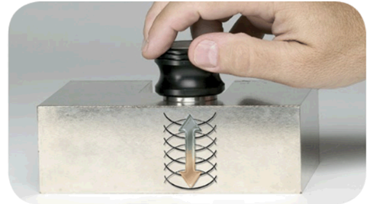
Longitudinal wave transducers – A106S and V109 (Pulse-echo Technique)
