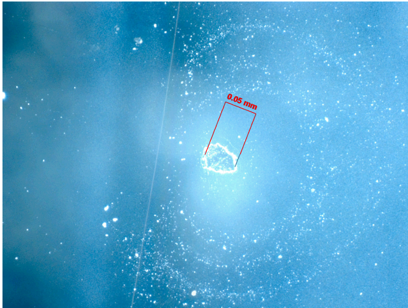
Laser spot profile on CL-20 film 50 \mu\text{m} film spot
