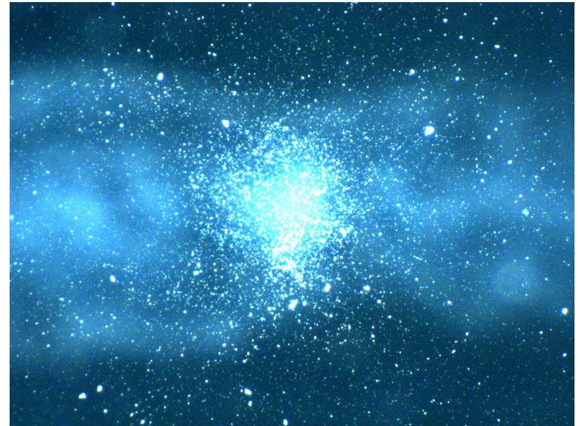
Printed CL-20 particles ~100 \mu\text{m} particle distribution
