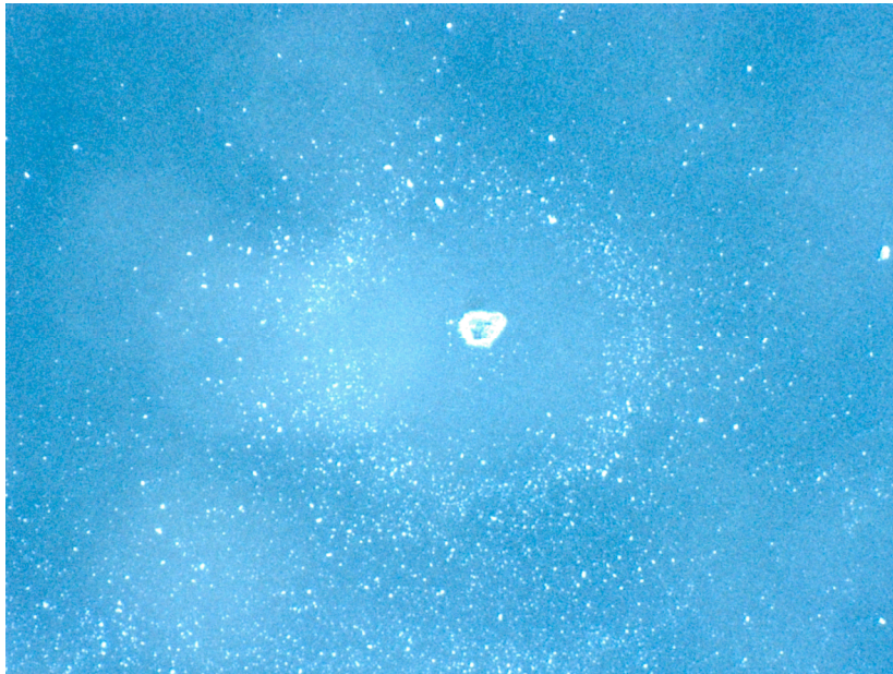
Laser spot profile on CL-20 film 17 \mu\text{m} film spot size
