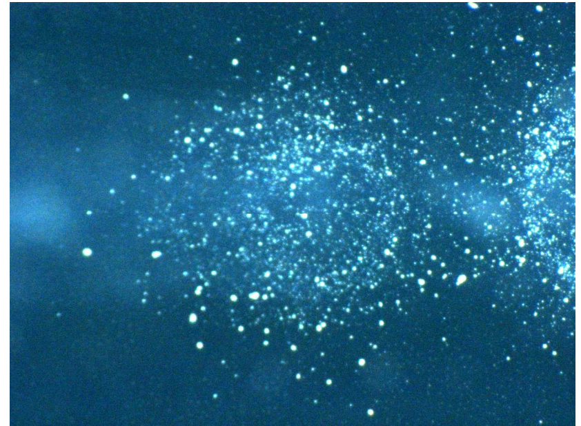
Printed CL-20 particles ~70 \mu\text{m} particle distribution
