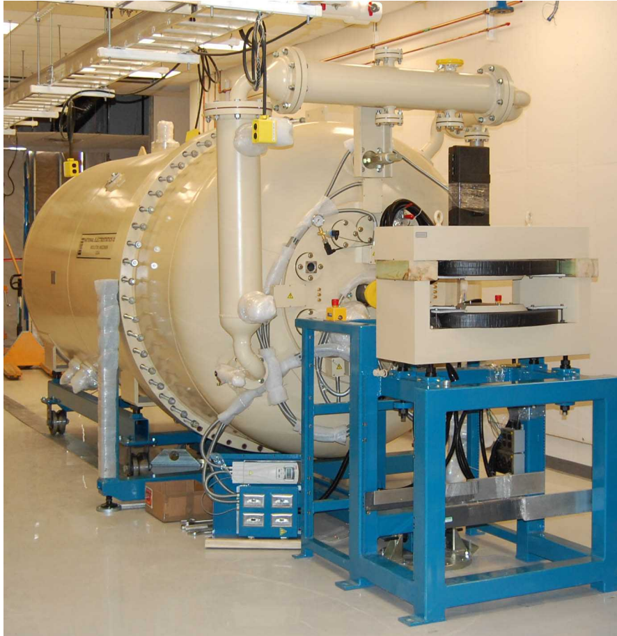
3MV single-ended NEC Pelletron being installed. Can maintain \pm 100V on terminal
