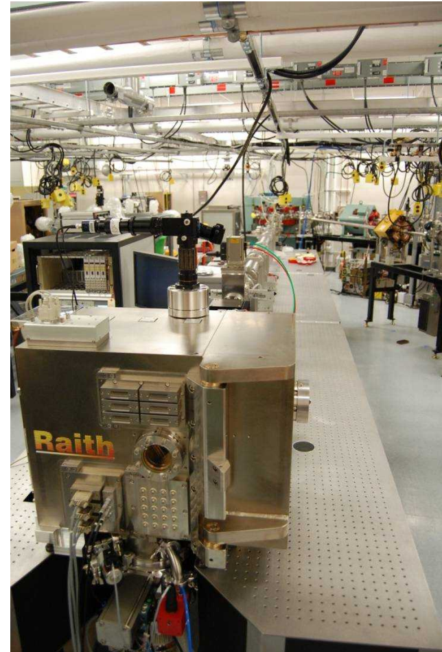
uBEAM line – 1\mu m spot for IBA, 200nm spot for SEU, nm resolution stage.
