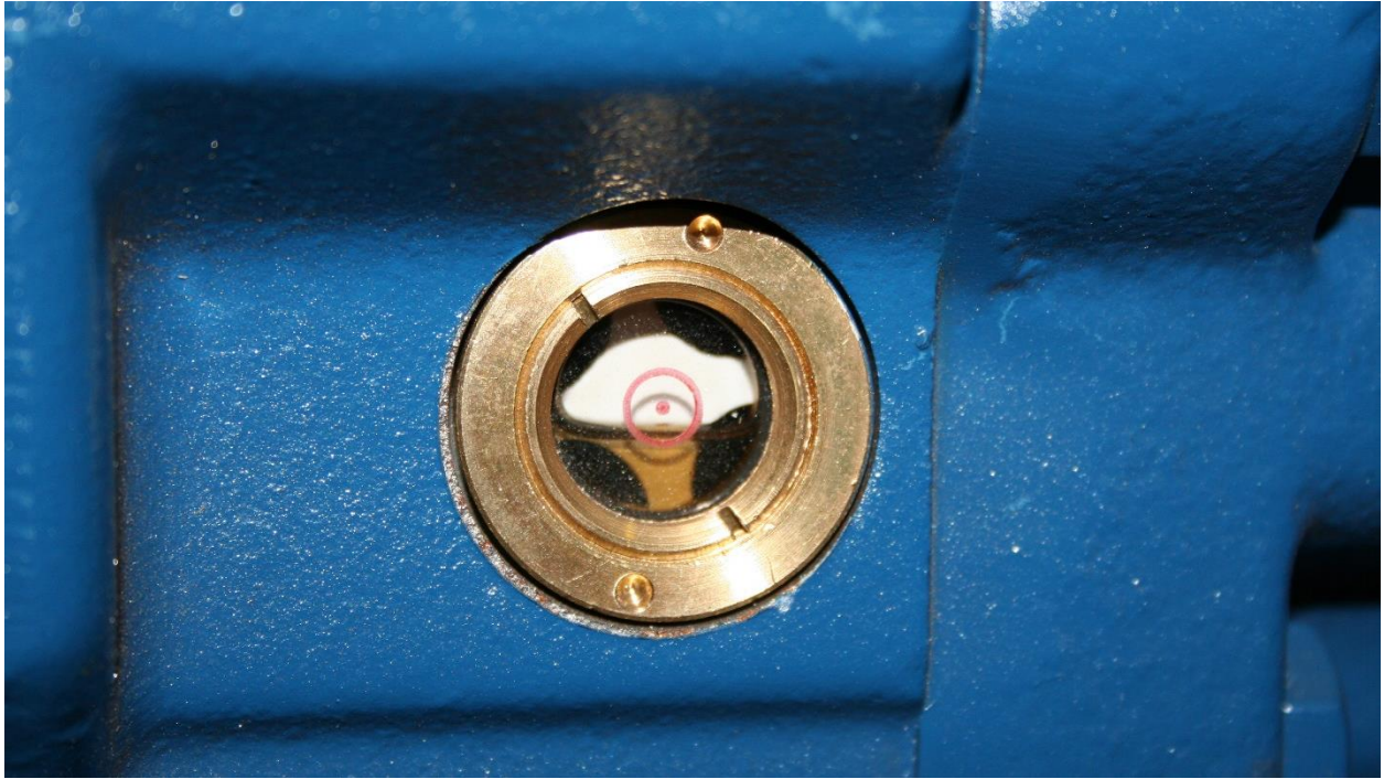
Figure B9. Oil level sight glass, showing some loss.
