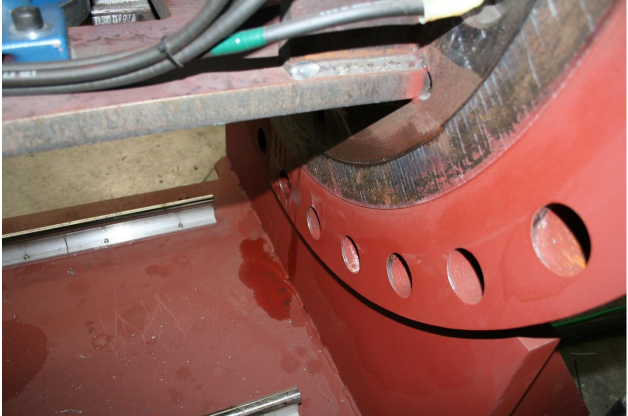
Figure B11. Oil on the vessel bulkhead, and dripping to the platform below after opening the tank.
