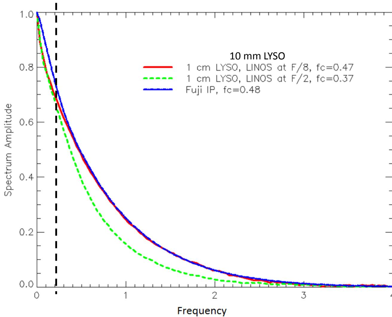
Low-frequency “tile glow” affect the scintillator similarly regardless of F-number. High frequency is affected more by optical blur which changes with F-number.
