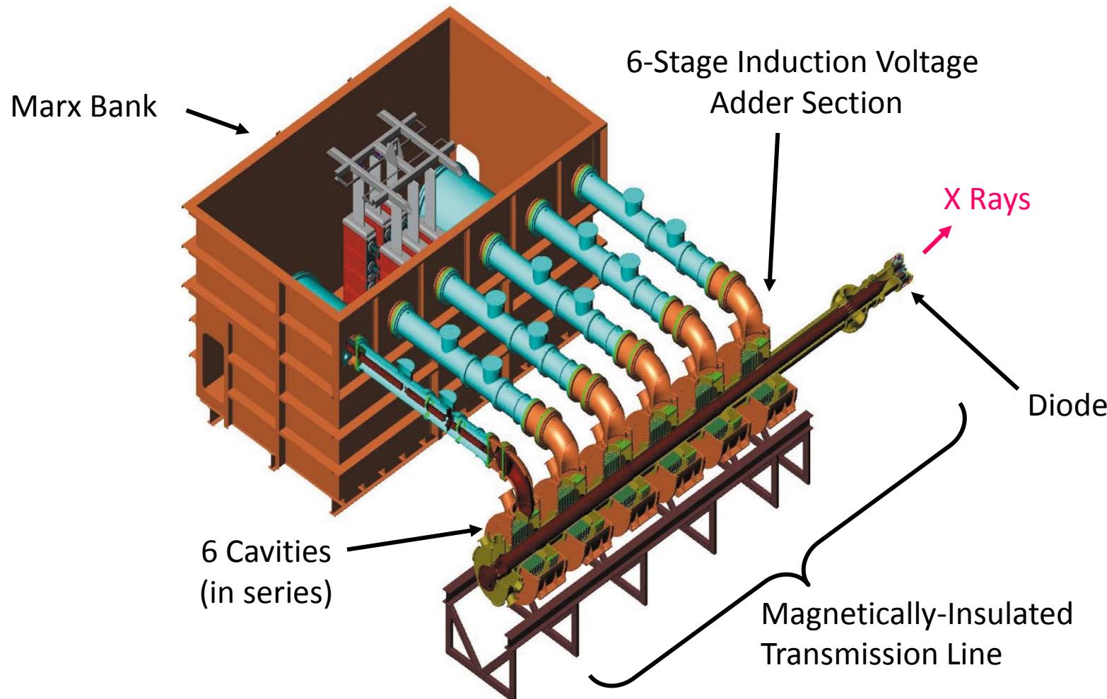
**RITS-6 is a 8-12\* MV Marx driven six-stage Inductive Voltage Adder (IVA) capable of driving a variety of flash x-ray radiography diode configurations (by my count around half-dozen different “diodes”)**
