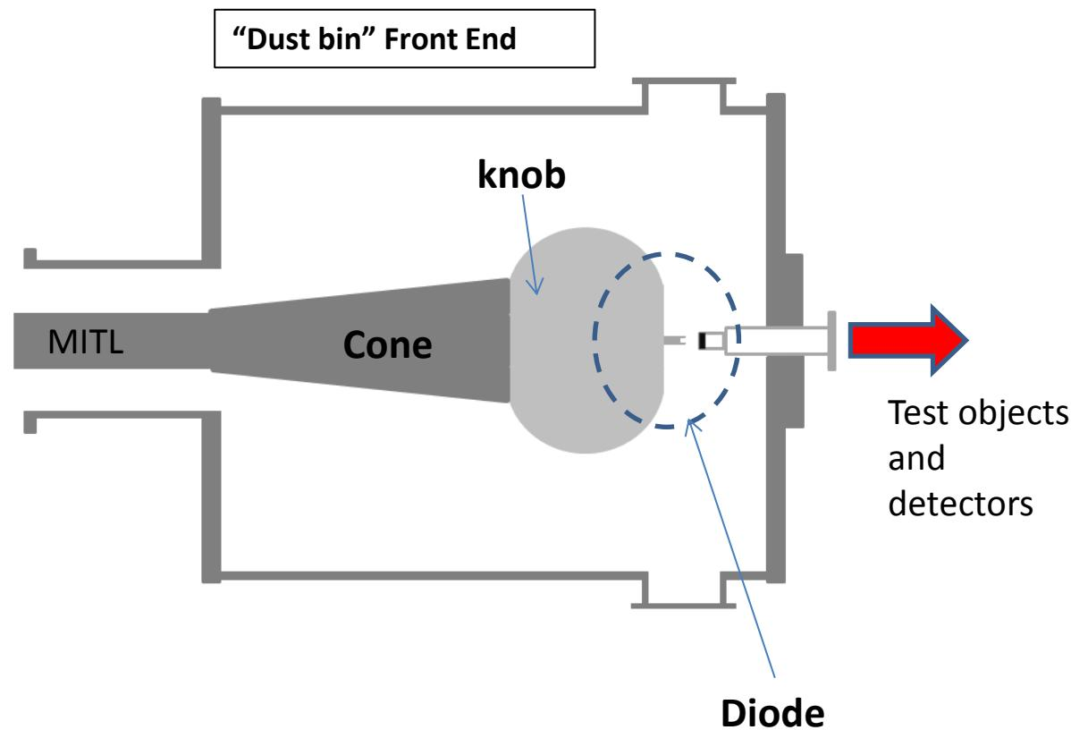
\*Traditionally the maximum voltage is changed by changing the MITL inner conductor. Over the last six months we have operated the machine as low as 2 MV by different operating points on the Marx generator and PFLs.
