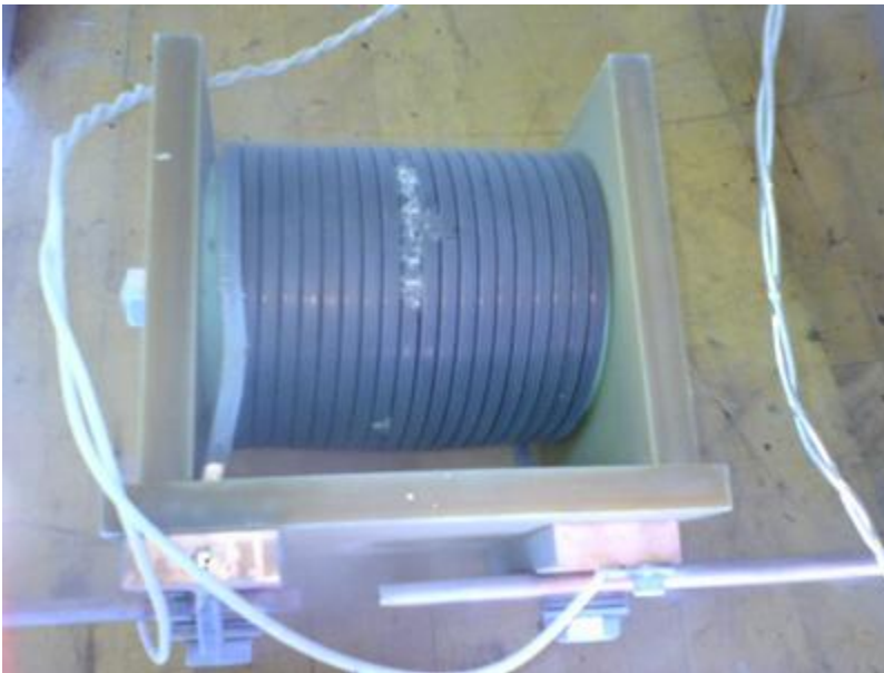
Figure 30: Shunt coil without overbanding with indications of insulation damage after pulsed current loading of ~ 35 kA. Coil has just been removed from LN2 bath.
