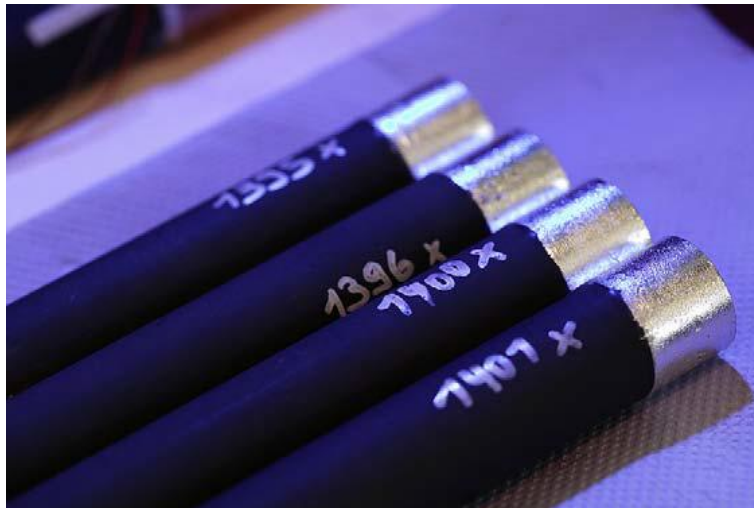
Figure 4: Examples of some of the BSCCO2212 MCP elements used in the Phase 1 work. The black part is the BSCCO2212 HTS material with silver end caps.
