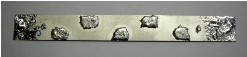
Figure 16 Indium “dots” test sample – 12 mm wide with 5 indium dots placed along tape. Current and voltage tap connections are also located on each end.
