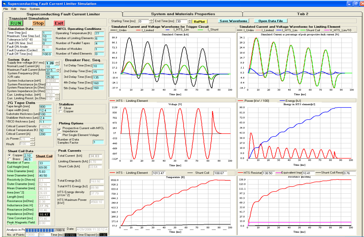
Figure 22 Example of the parametric modeling tool developed for evaluating the SFCL under a range of operating parameters. Output includes plots of the voltage and current traces for the superconductor elements and shunt coils, temperature rise and fault current reduction.
