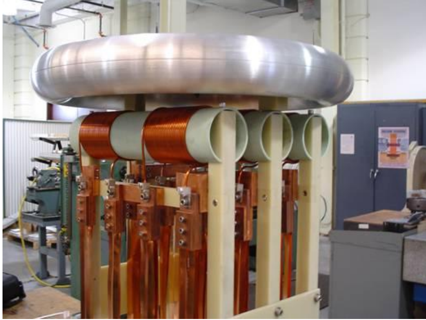
Figure 39: Intermediate meander path module construction with voltage rings (top and bottom). Shunt coils are present between the meander path and voltage rings.
