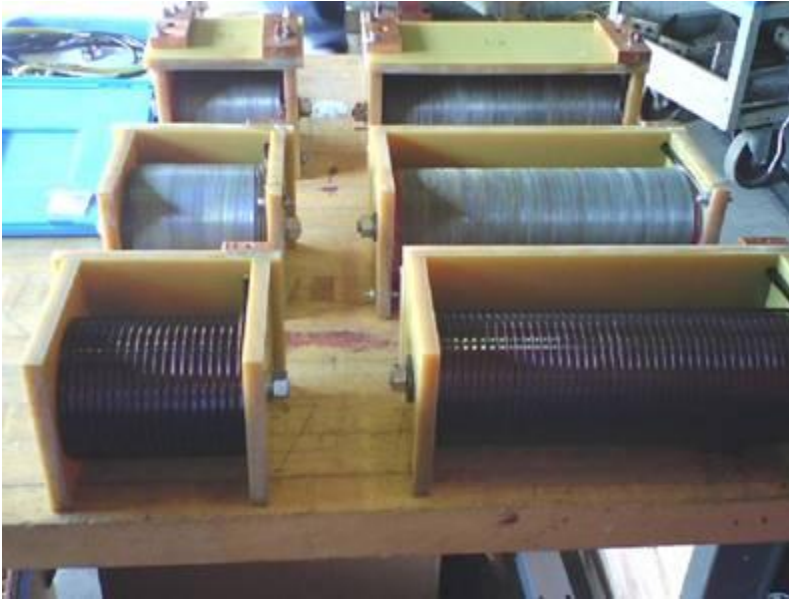
Figure 29: Six demonstration shunt coils, 4 with stainless steel overbanding (rear) and two without overbanding (front).
