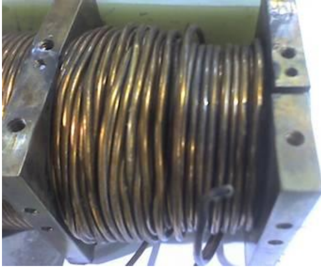
Figure 27: Photo of an early shunt coil that failed during a fault transient test. The coil was subjected to very high hoop stresses and thermal loading during the test, resulting in a failure of the copper windings.
