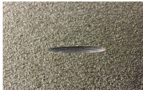
Grinder Disk Grove *Gouge or deep scratch
