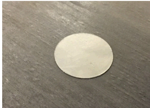
Grafoil insert *Tight delamination
