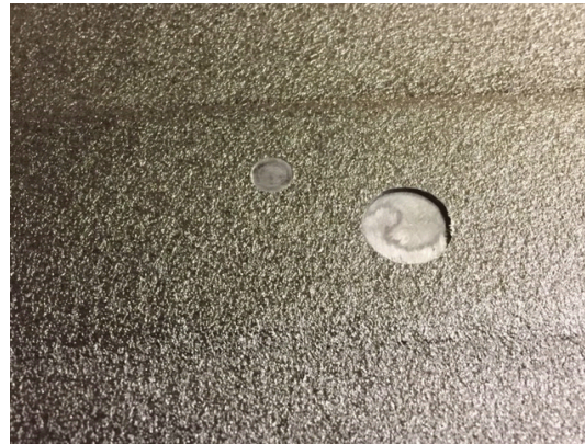
Flat bottom holes *Significant delamination
