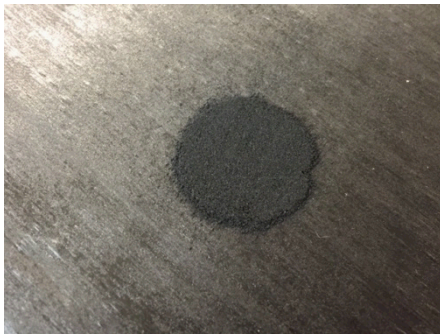
Carbospheres *Localized porosity
