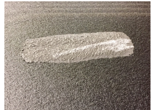
Sealant *Raised material, not a flaw
