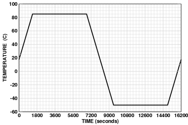
Figure 4. Accelerated aging cycle: 90 minute holds, temperature minimum -50°C; temperature maximum, 85°C.
