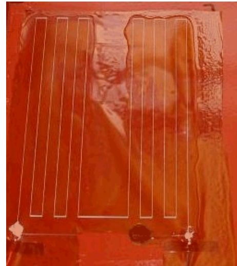
Ag traces on powdercoat w/overcoat
