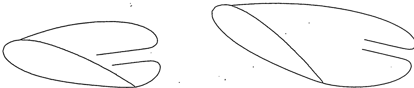
Figure 13 R-J flow past an inclined airfoil with fixed separation points.
