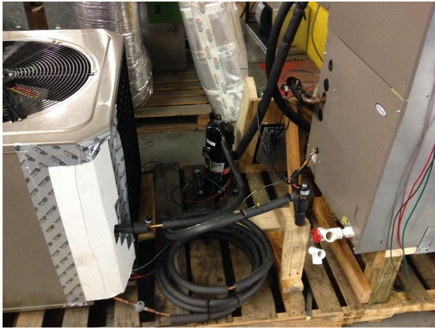
Figure 5: First prototype, cooling only, single variable speed compressor
