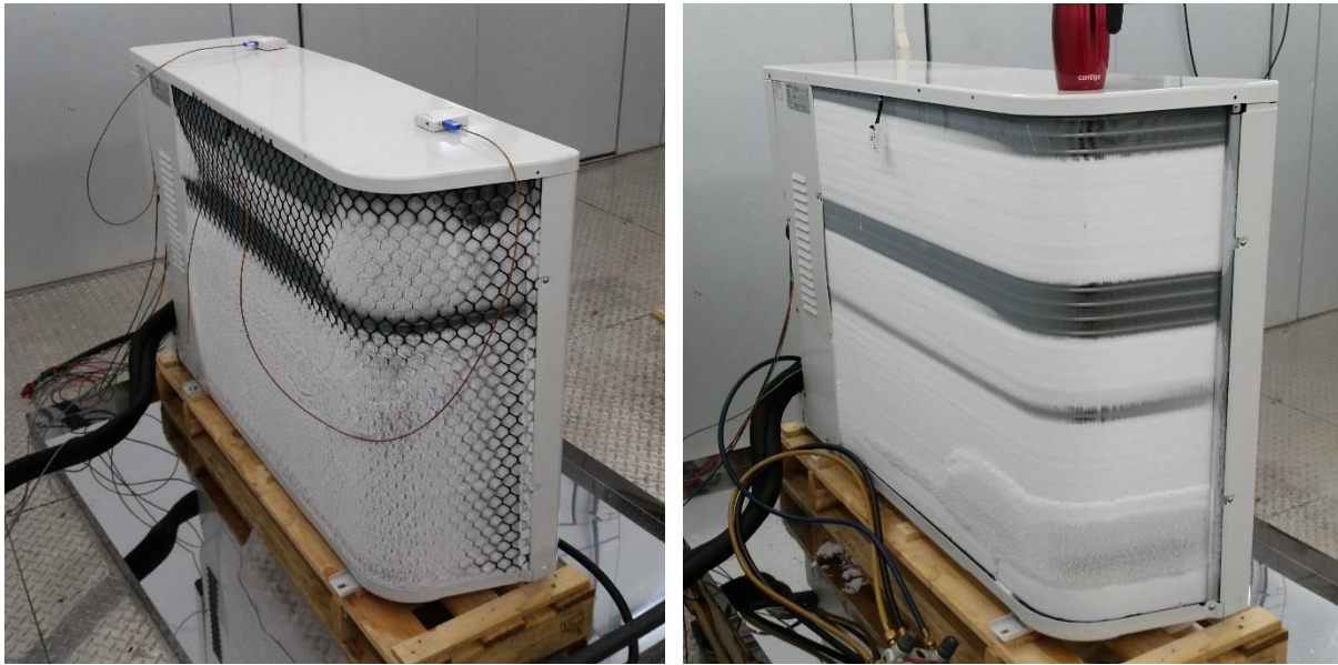
Figure 16: Defrost with fin protector screen (left) and without (right)
