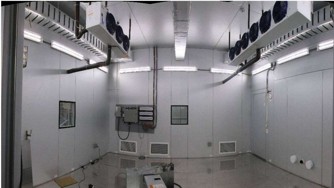
Figure 2: Outdoor test chamber (Chamber #3). Intermediate temperature refrigeration system is shown upper left. (Used to pull temperature down from 30°F to 10°F)
