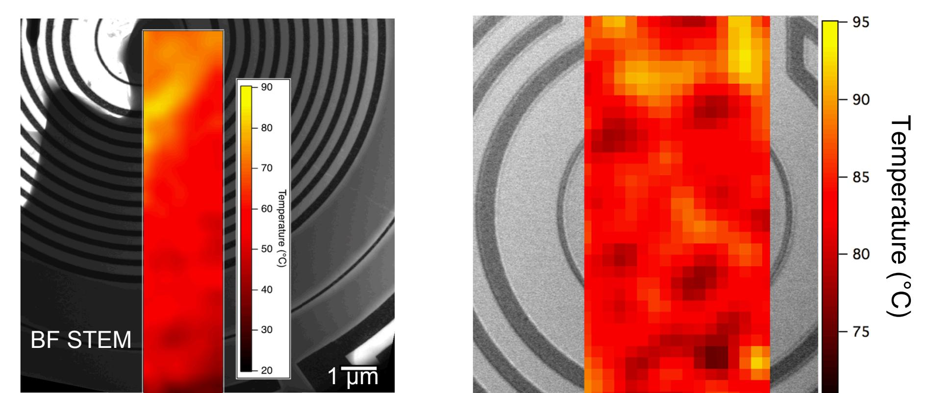
Temperature fairly uniform in center, given a measurement technique accuracy of order 10 °C.
