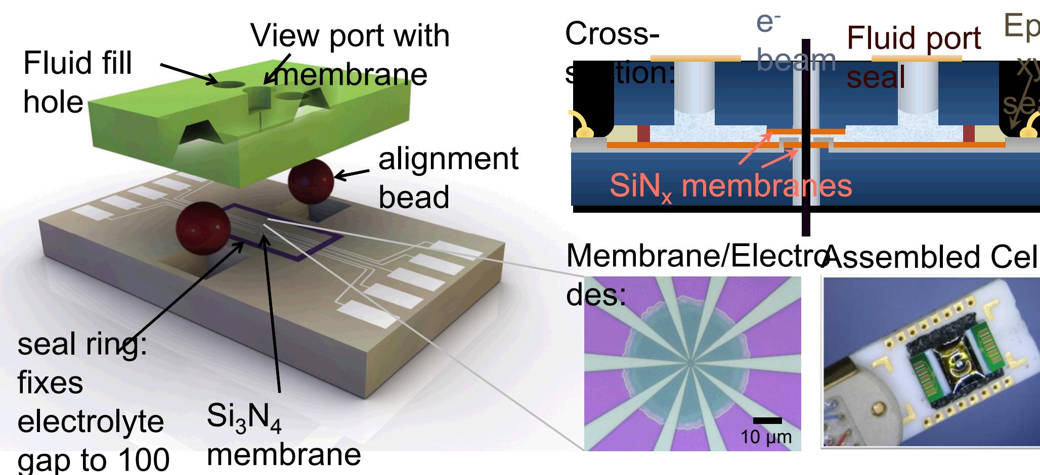
Materials of study in liquid or on electrodes; cell filled with ~100-nm thick liquid layer.
