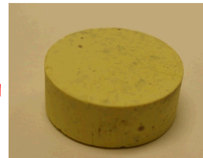
Glass/AgI-MOR pellet sintered to high density at 550°C.
