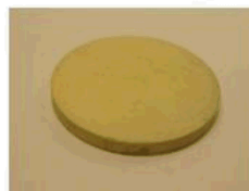
50 wt% AgI/50 wt% Glass, 500° C for 3 hr
