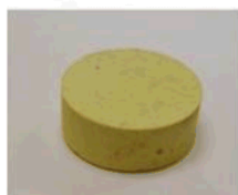
50 wt% AgI/50 wt% Glass 500° C for 3 hr
