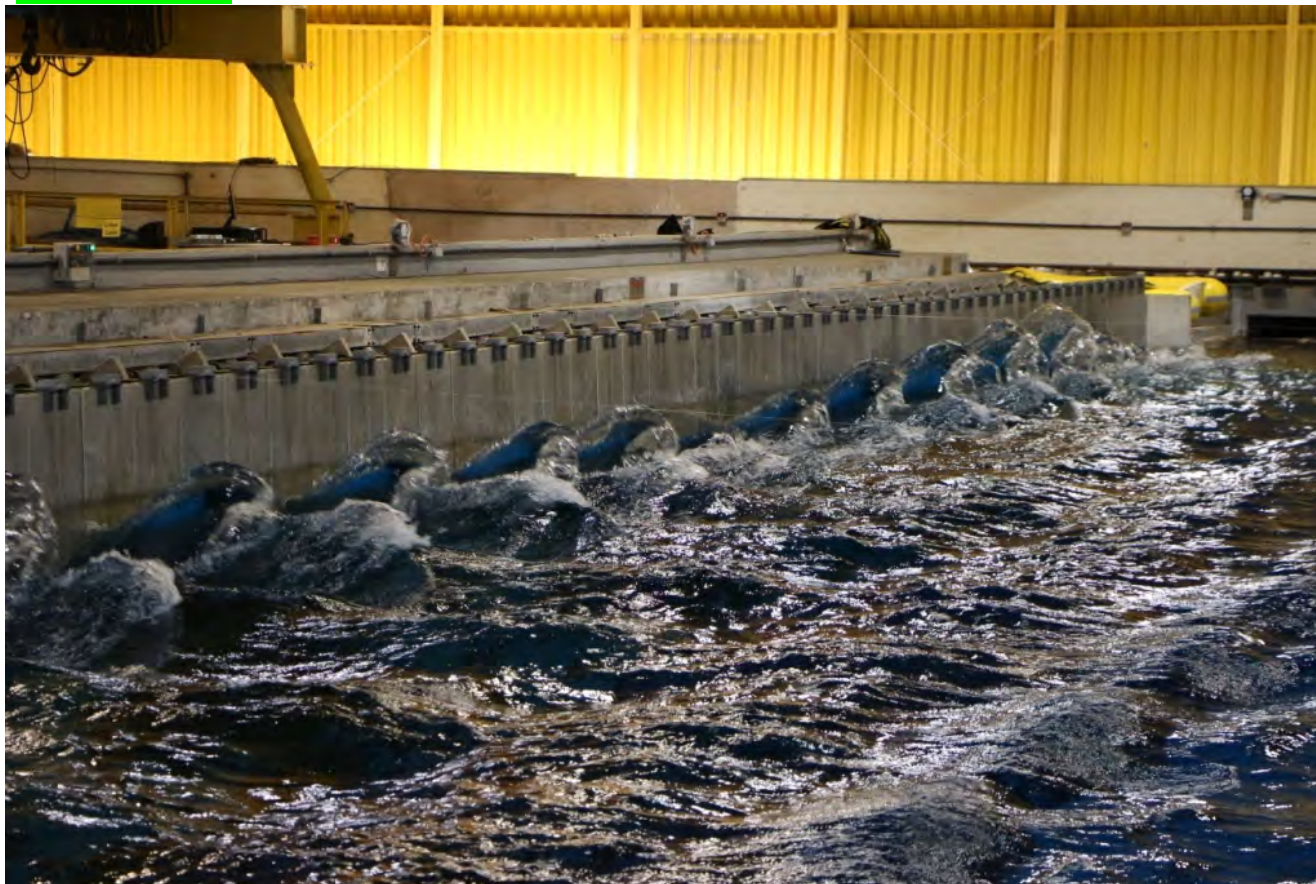
Figure 5-40 - Transverse Waves Generated on the 10 year Sea Wave
