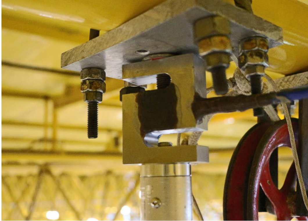
Figure 4-4. Top connection of CWP for impulse tests.
