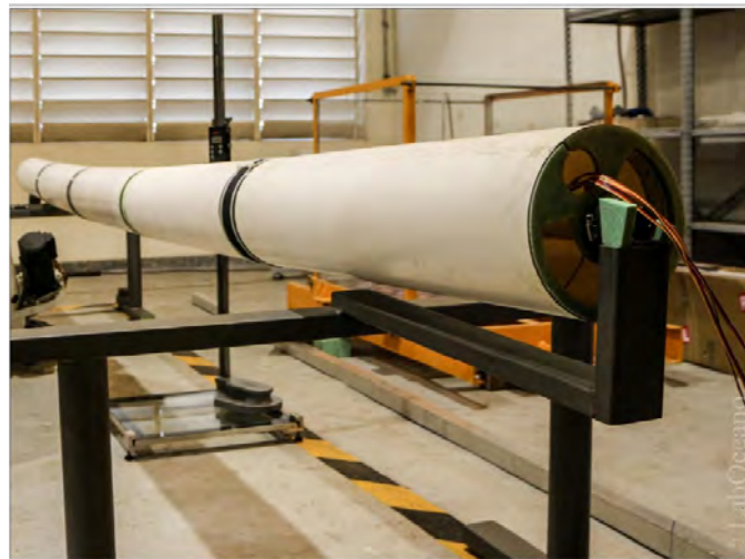
Figure 2-7 Setup for Pipe Bending Calibration
