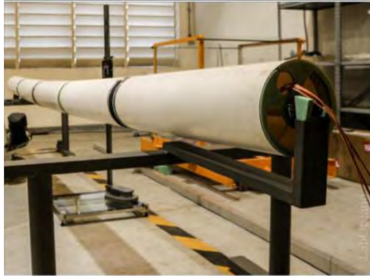
Figure 23 Setup for Pipe Bending Calibration
