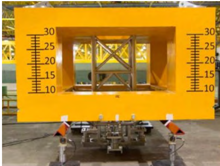
Figure 21 Semi-Submersible Model with CWP Support Frame
