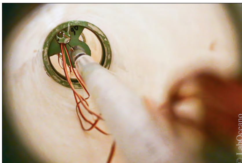
Figure 5-11 - Strain Gage Installation
