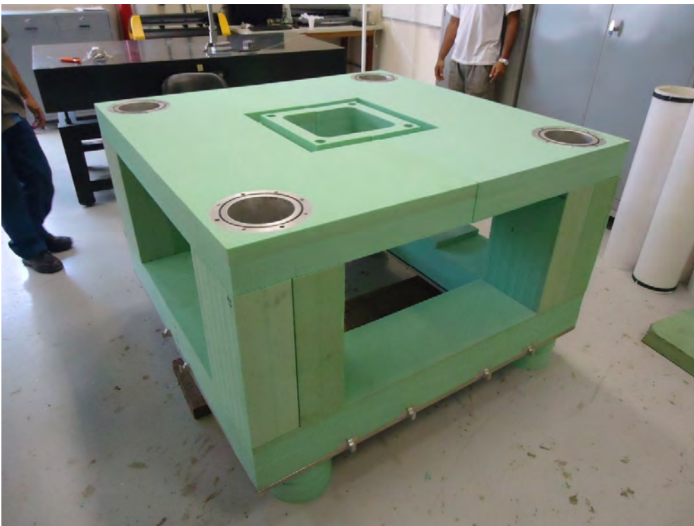
Figure 3-7 - Semi-Submersible PVC Foam Filling
