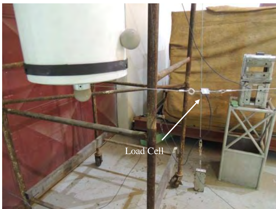
Figure 4-5. Pulling line and load cell for static offset test
