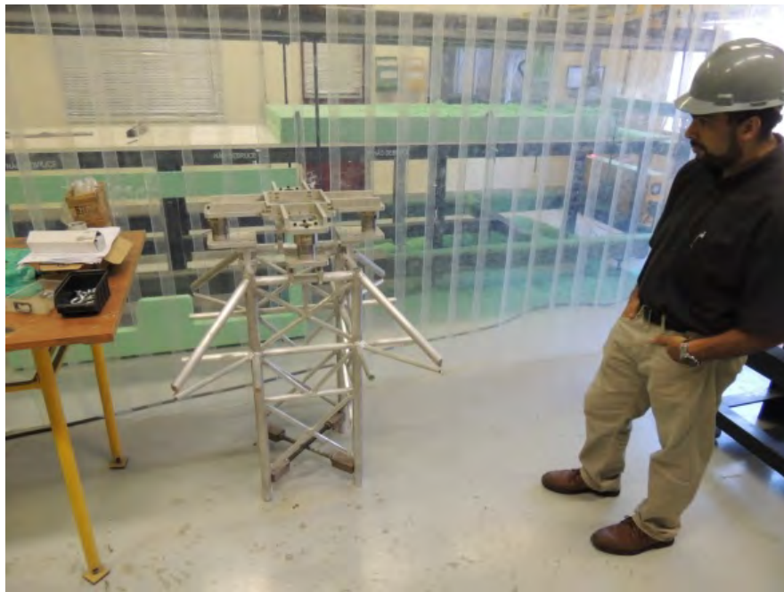
Figure 3-9. Truss and gimbal support showing the four load cell dynamometer design.
