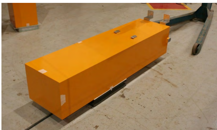
Figure 3-29. Remora X and Z CG Measurement
