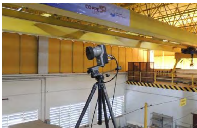
Figure 4-2 Optical tracking camera measuring displacement of vibrating CWP
