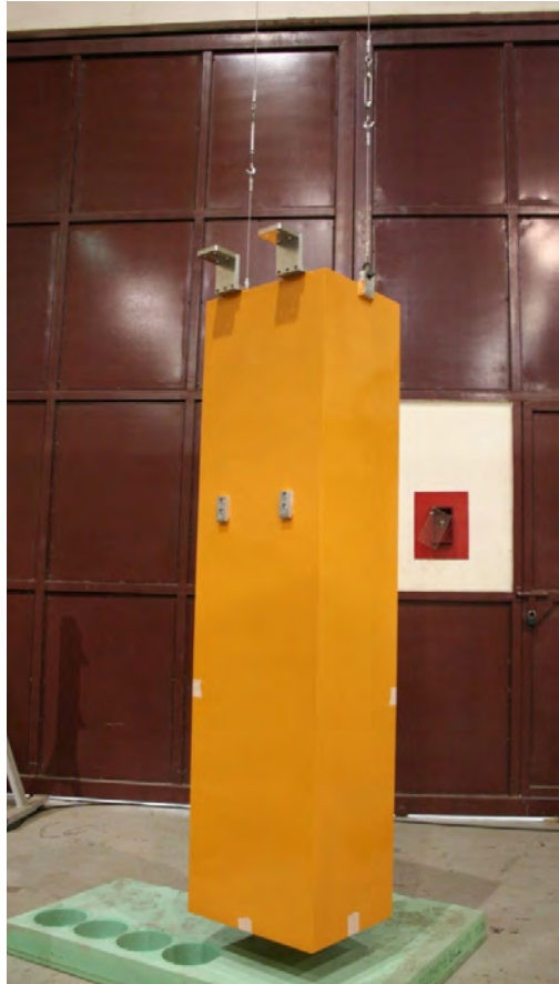
Figure 3-32. Remora Izz Moment of Inertia Bifilar Measurement
