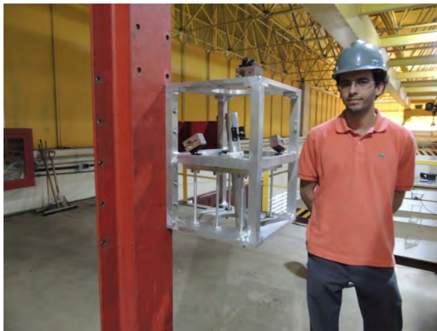
Figure 3-6. Gimbal model with zero stiffness
