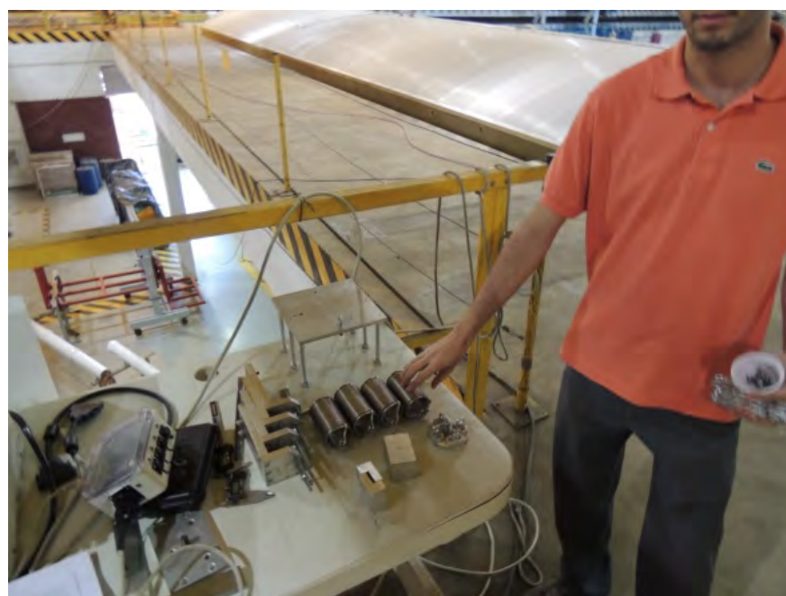
Figure 3-7. Spring and bracket components for gimbal with operational stiffness.
