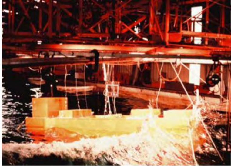
Figure 13 1:30 Scale Model of 40 MW OTEC Plant, 1982 [12]
