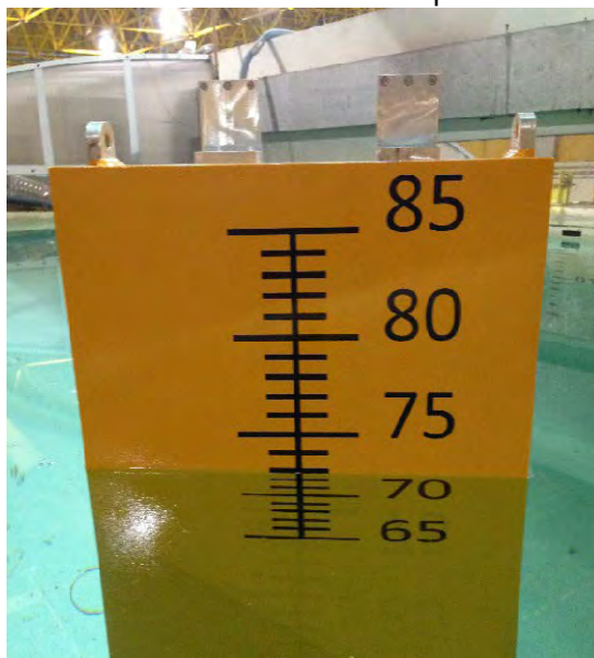
Figure 3-34. Remora Draft and Natural Period Check
