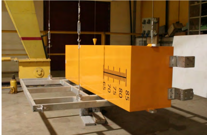
Figure 3-30. Remora I_{xx} Moment of Inertia Trifilar Measurement
