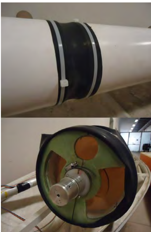
Figure 3-5. Photographs showing assembled CWP section with rubber sleeve and core connection.
