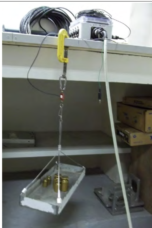
Figure 5-19 - Load Cell Calibration
