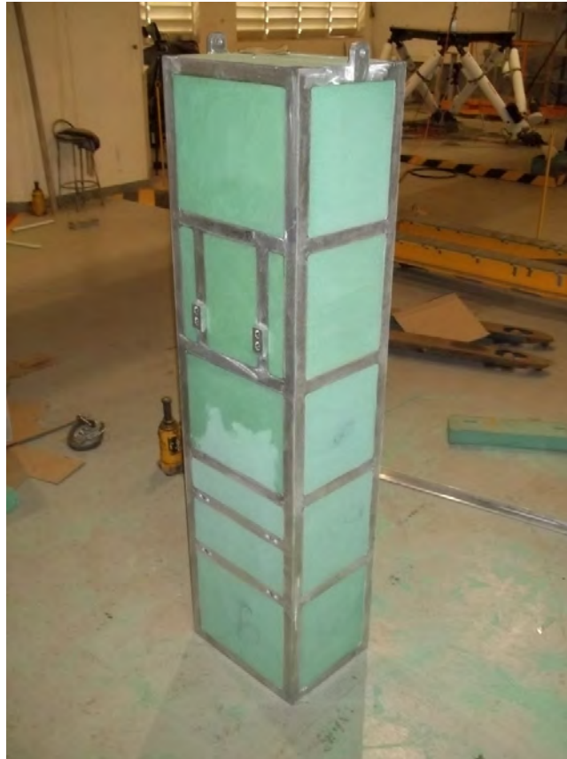
Figure 3-22 - Remora PVC Foam Filling
