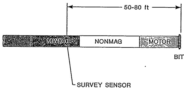
Figure 1. Conventional MWD Drill-String Location
