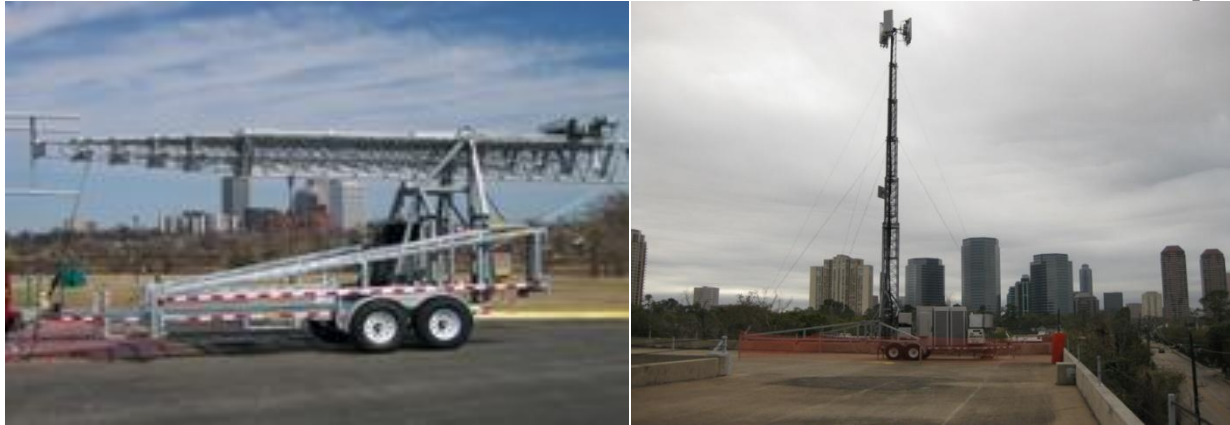
FIGURE 22: ALLTECH 106 FOOT TOWER BEING TRANSPORTED (RIGHT) AND IN USE BUT NOT FULLY EXTENDED (LEFT)
