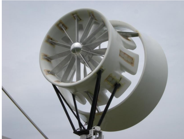
Figure 3, Briza Prototype MEWT
