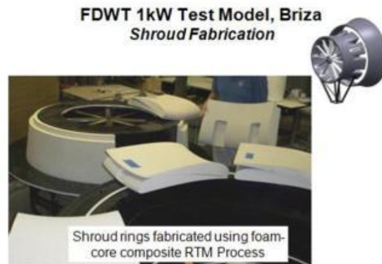
Figure 14: Composite Shroud Fabrication
