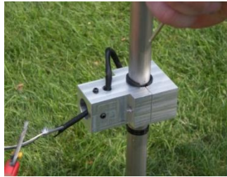
Figure 11, New Bracket for anemometer
