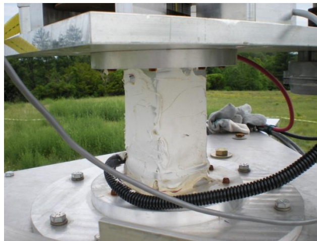
Figure 2: Load Beam Instrumented with Strain Gages
