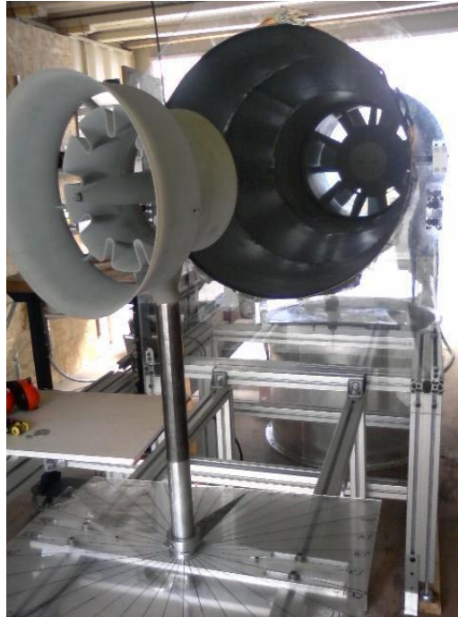
Figure 56: Load Balance and Yaw Measurement System
