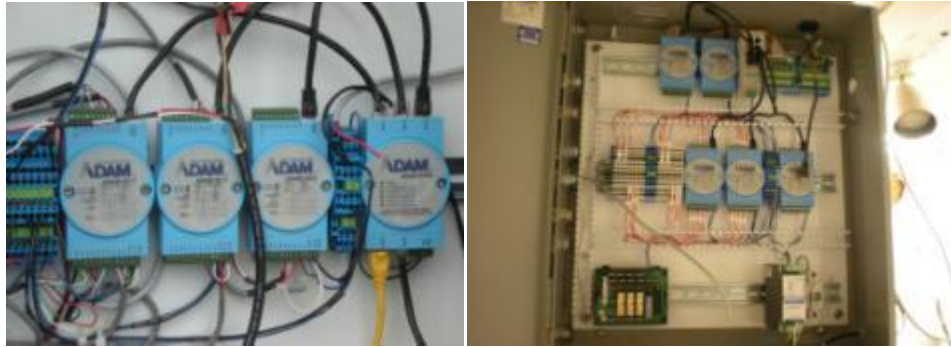
Figure 21: Data Acquisition System Modules for Analog to Digital Conversion
