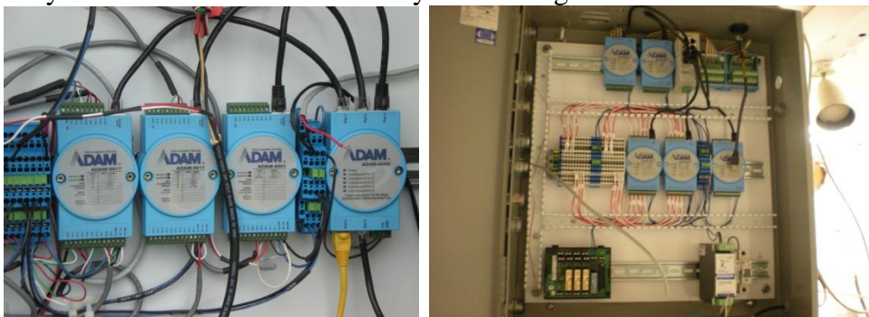
Figure 21, ADAM modules in blue at Briza, Figure 22, ADAM modules in ME DAS
