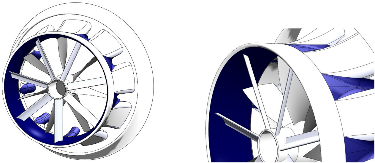
FIGURE 26: ANGLED VIEW OF C481 WITH A STATOR ROTOR (LEFT) AND CLOSE-UP OF STATOR ROTOR (RIGHT)
