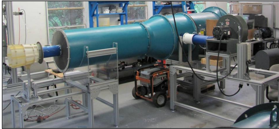
Figure 51: Dual Flow Wind Tunnel Test Setup
