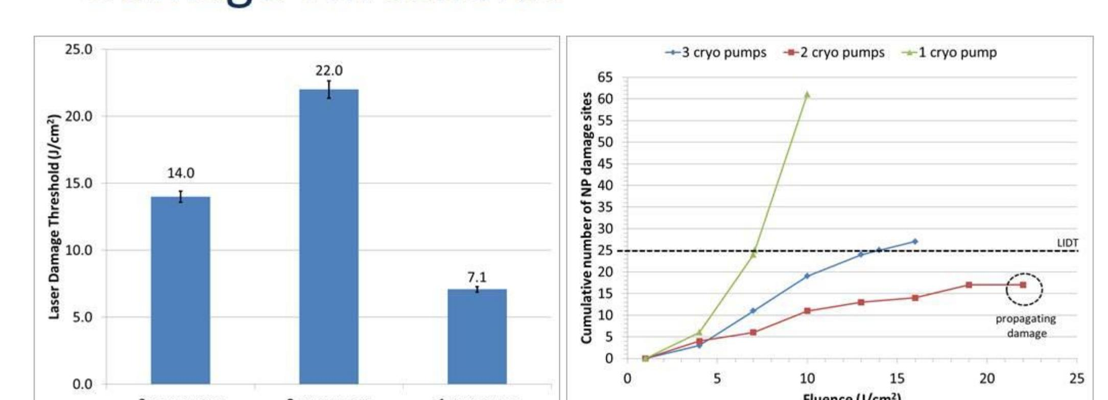
The highest laser damage threshold was achieved with 2 cryo pumps rather than 3. The coating deposited with 3 cryo pumps reached its damage threshold due to the accumulation of >25 non-propagating defects – the substrate may not have been cleaned as thoroughly as it could have been.
