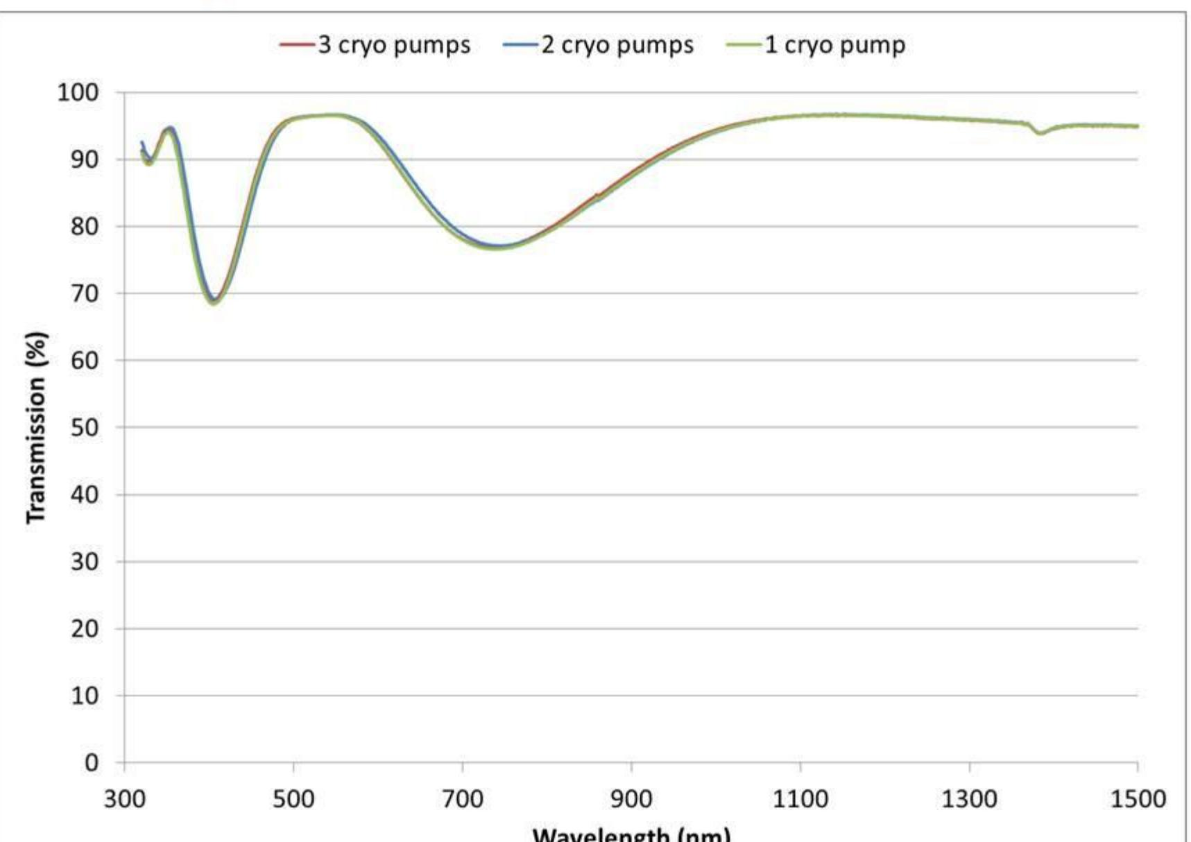
Transmission scans acquired ~1 month after deposition to account for spectral shifts due to aging 4
