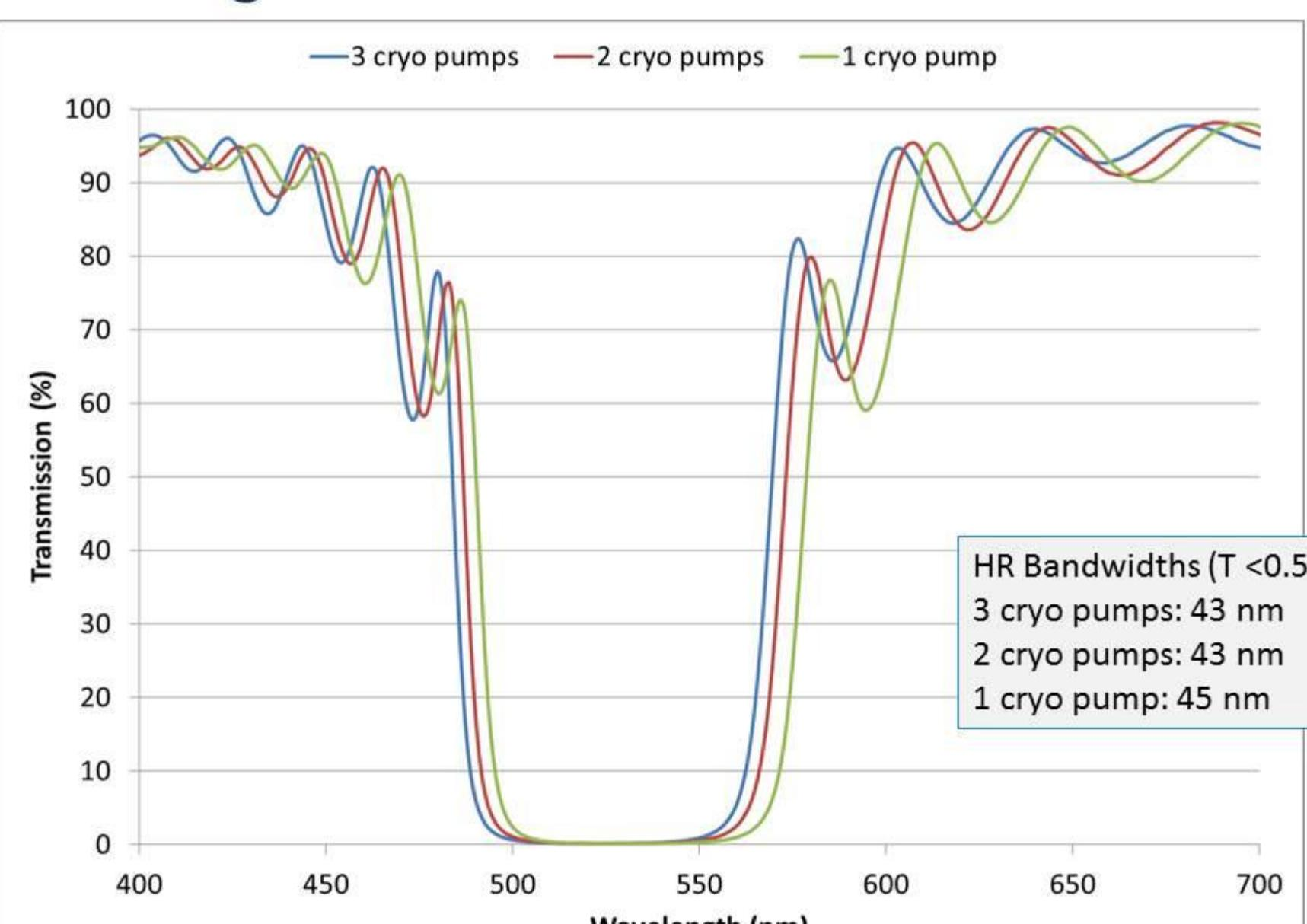
Transmission scans acquired ~1 month after deposition to account for spectral shifts due to aging 5
