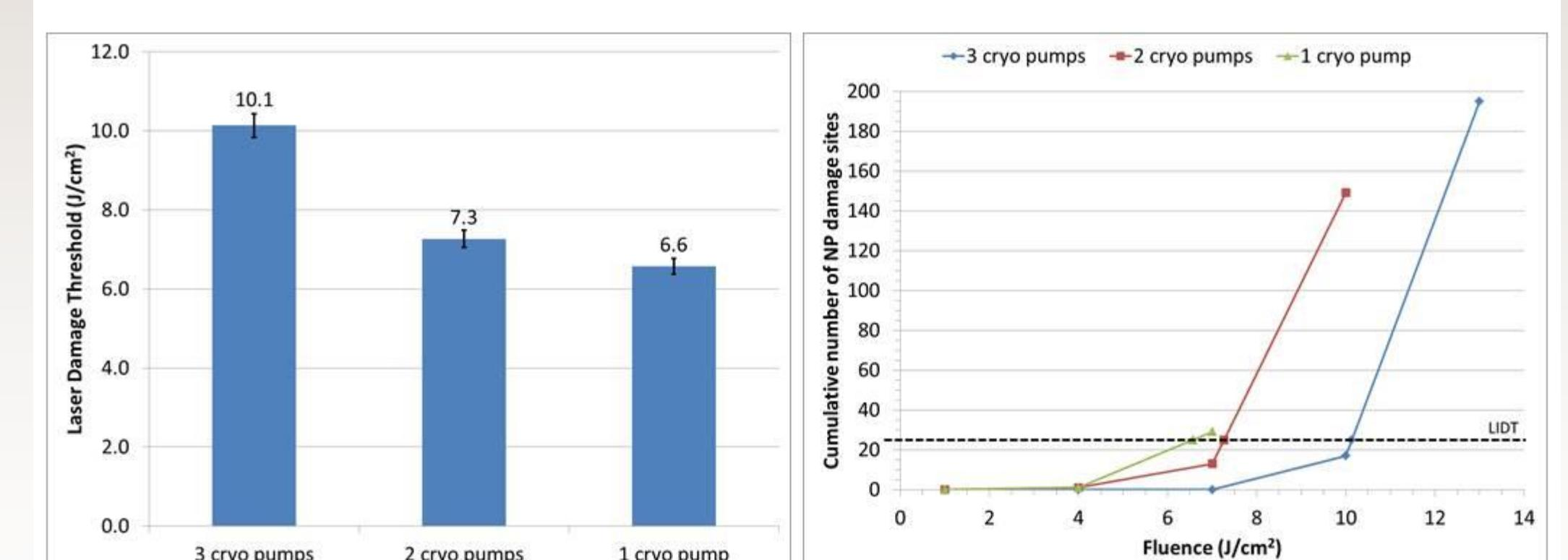
Laser damage thresholds decline with fewer cryo pumps operating during the coating deposition.
