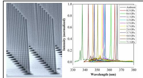
Fig. 3: Left panel shows GaN nanowires with controlled dimensions fabricated by two-step dry + wet top-down approach. Right panel shows lasing spectra of GaN nanowires under hydrostatic pressure.
