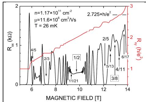
Fig. 1: Magneto-resistance  $R_{xx}$  and Hall resistance  $R_{xy}$ . A quantized plateau is observed at  $v=4/11$ .
