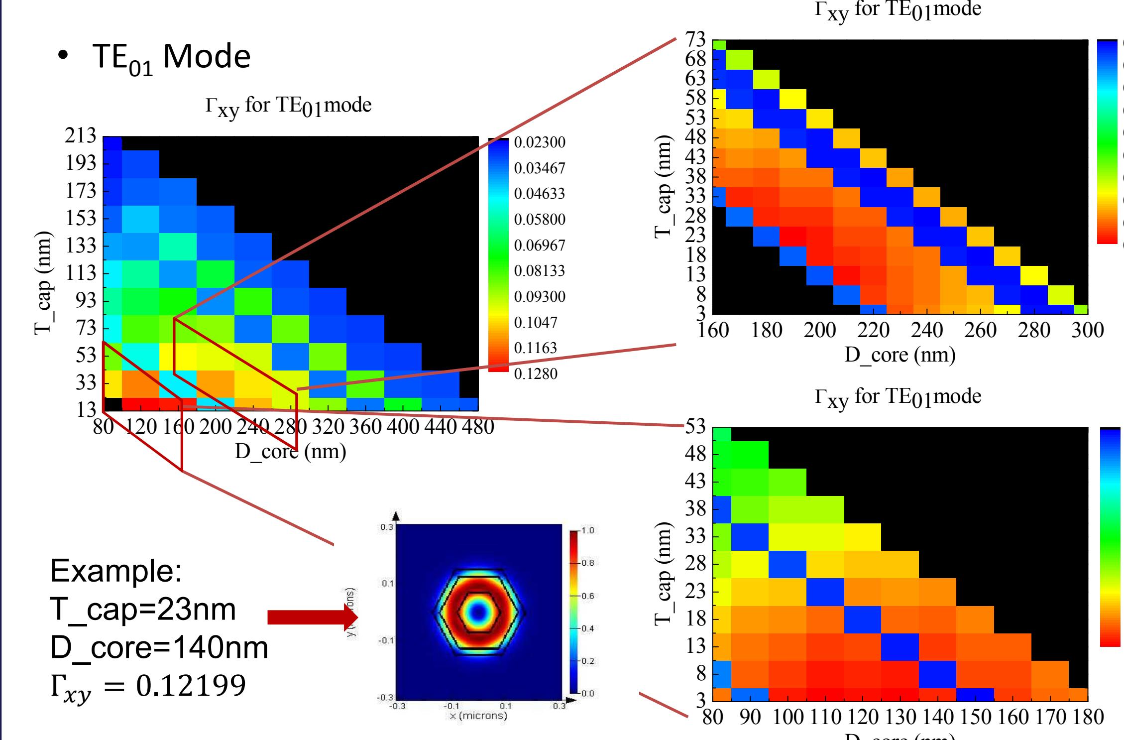
Simulation of transverse confinement factor ( $\Gamma_{xy}$ ) of TE<sub>01</sub> mode as a function of core diameter and shell thickness.  $\Gamma_{xy}$  varies from 12% to 2% with different structure design. This variation results in different lasing thresholds of the core-shell nanowire lasers.
