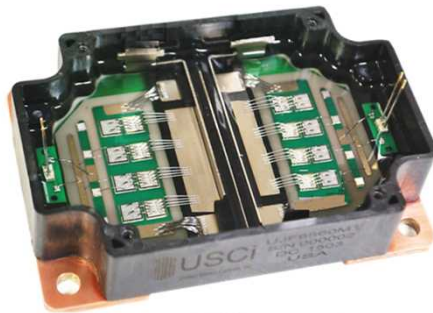
6.5kV 60A SiC JFET Half-Bridge Module
