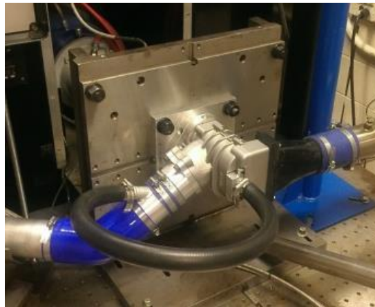
Figure 35: High Pressure Recirculation Setup
