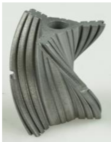
Figure 32: Additive Manufactured Aluminum Support Structure
