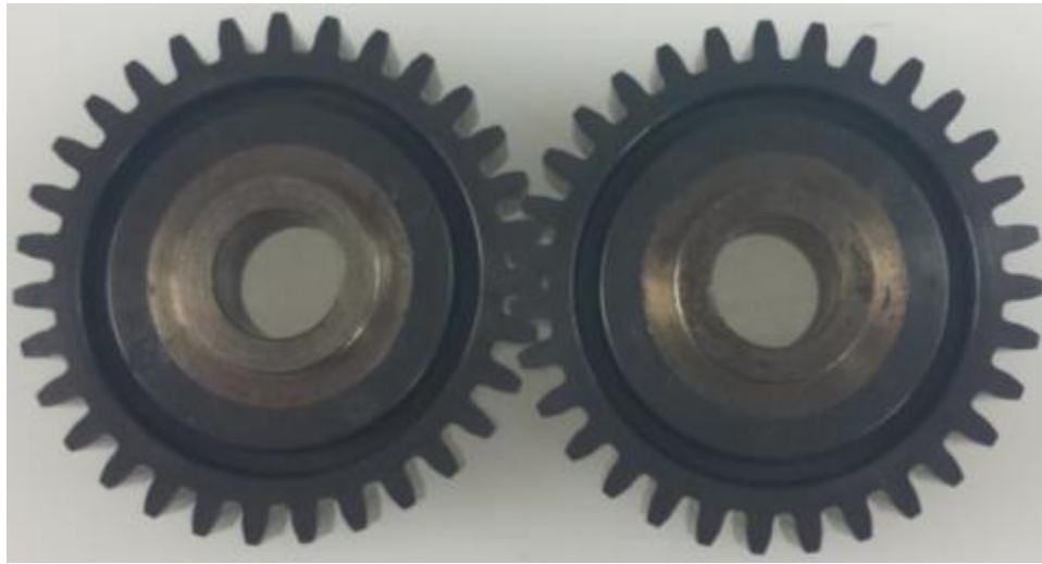
Figure 55: Plastic Expander Timing Gears
