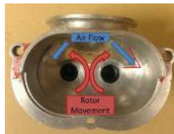
Figure 51: V250 Gen 1 Rotor Housing with Direct Air Flow Path
