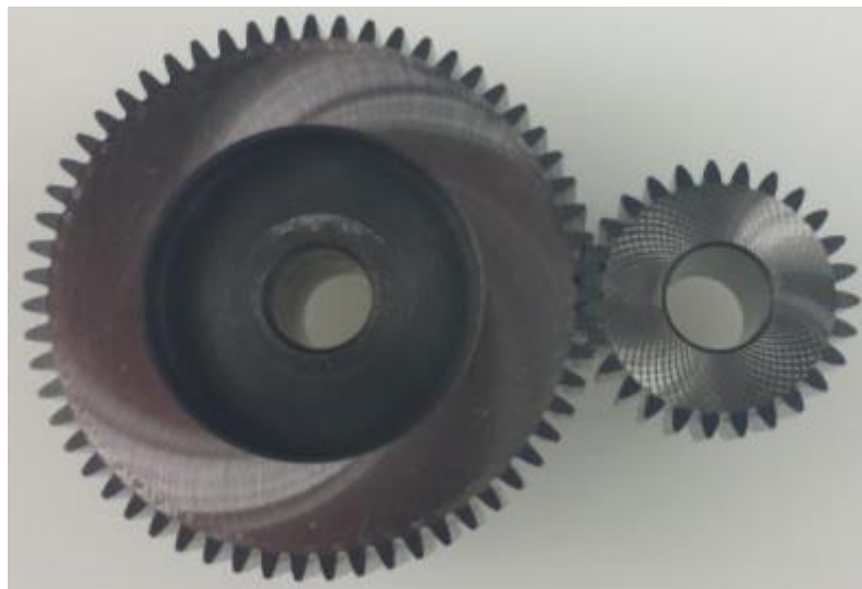
Figure 56: Steel Motor to Expander Step-Up Gears
