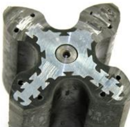
Figure 28: Rotor posttest (conditions 20,000 rpm at 110C). No failure and no indication of delamination. Scuff marks from contact with housing delamination from the aluminum support structure.
