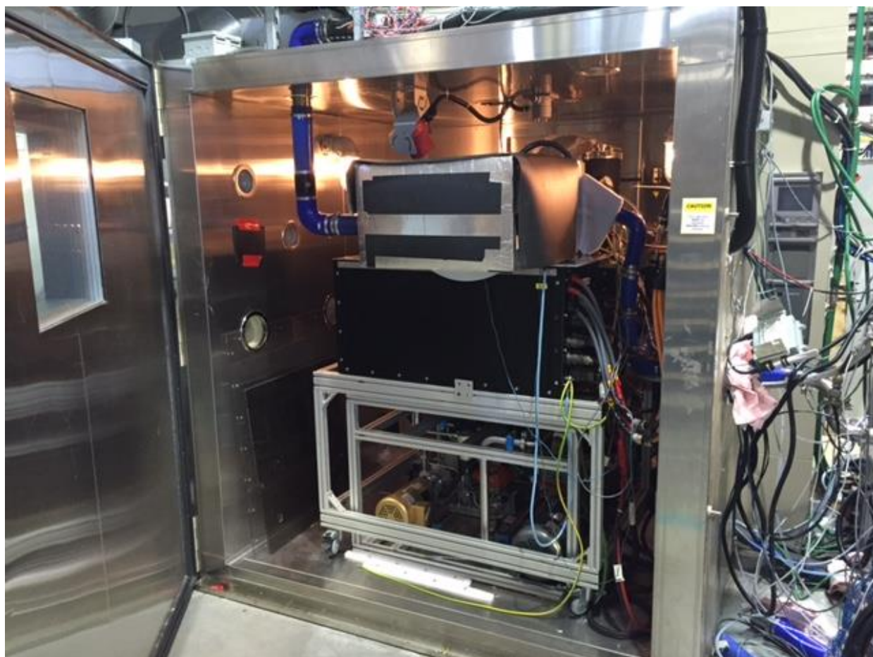
Figure 96: Ballard HD7 Module with Eaton Air Management System
