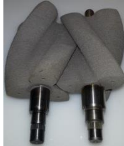
Figure 39: 3-Lobe Compressor Rotors
