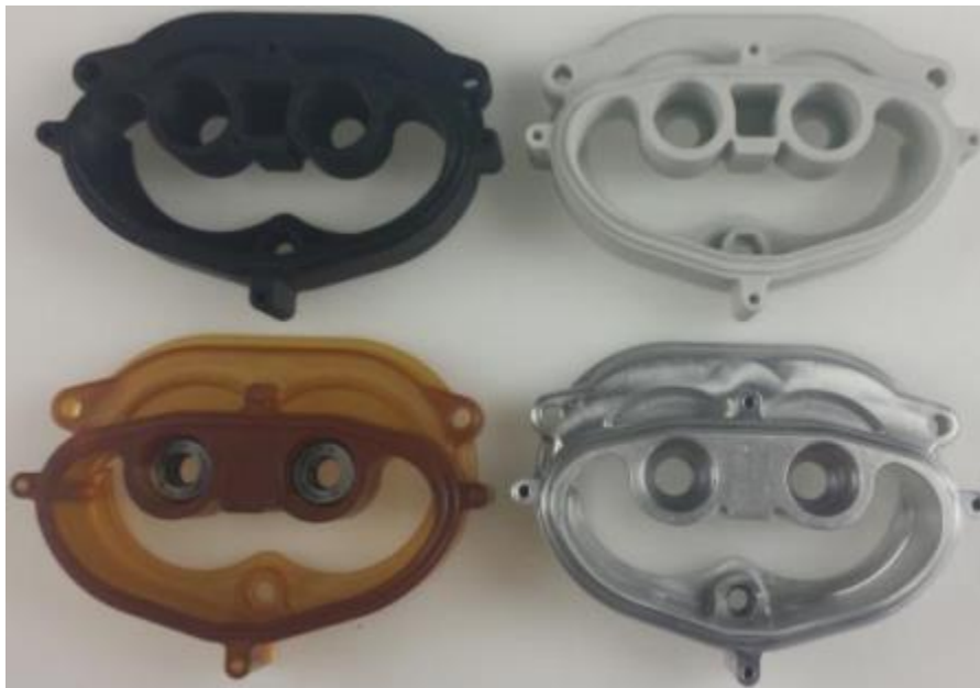
Figure 54: Expander Outlet Plates in Multiple Materials
