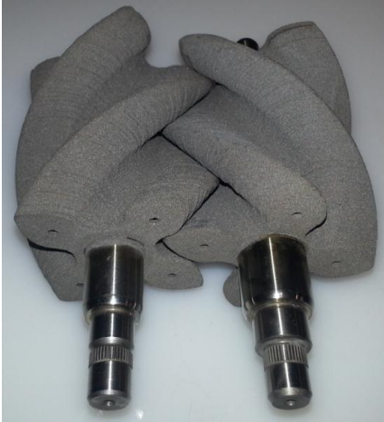
Figure 38: 4-Lobe Compressor Rotors
