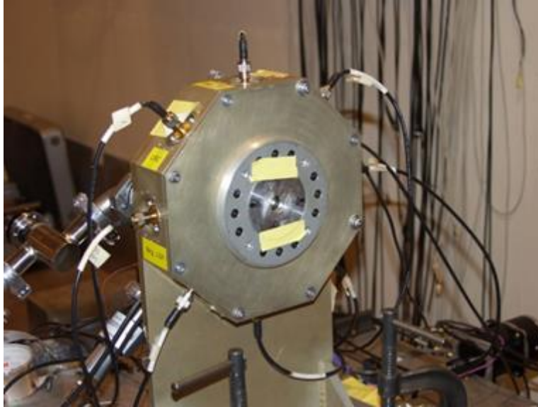
Figure 3. The vacuum experimental chamber with high voltage cables exiting through vacuum feed-through connectors.
