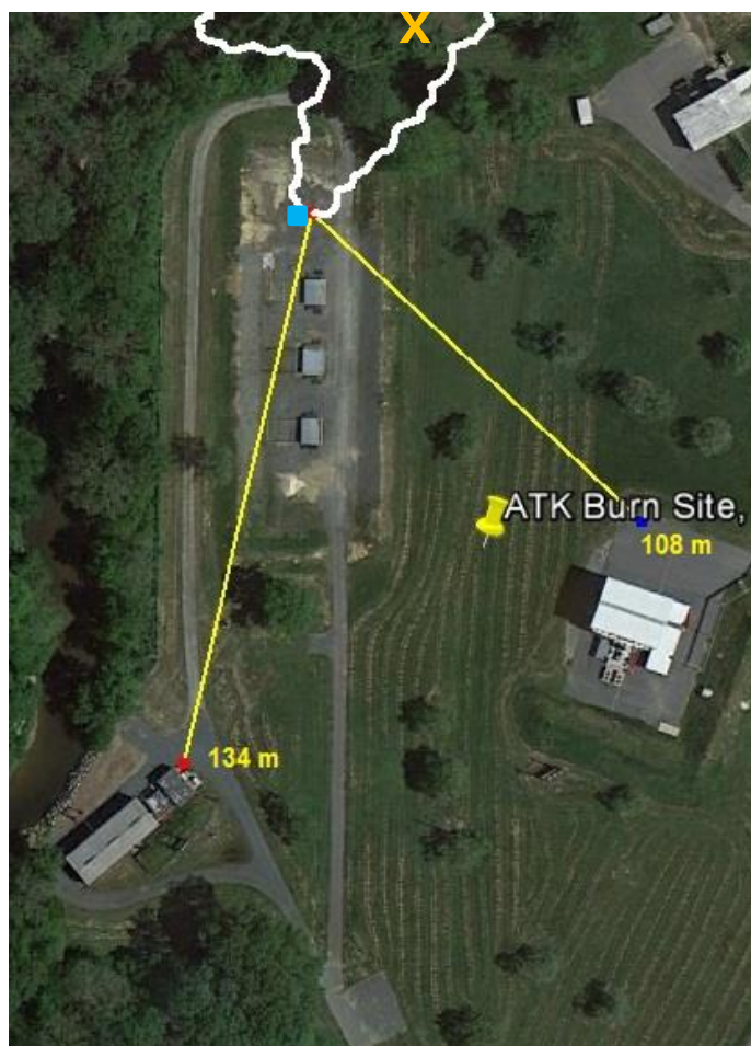
Figure 34. Aerial view of estimated plume extent at 1 min 13 sec into the burn on June 6, 2012.
