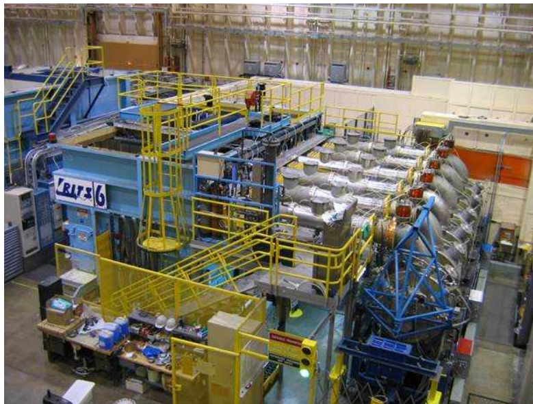
Figure 2. Photo of the RITS-6 accelerator. The diode is at the end of the accelerator towards the upper-right behind a shield wall.
