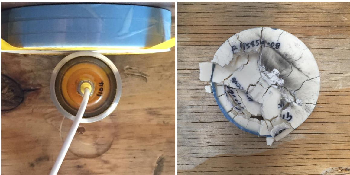
Figure 8. Direct contact test and resulting damage.
