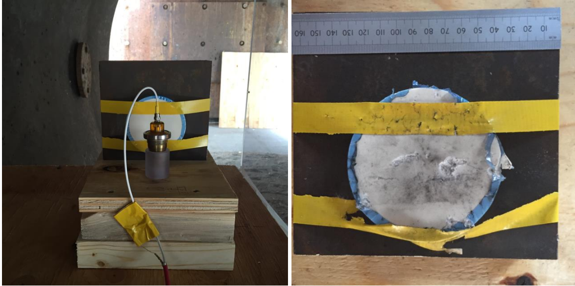
Figure 7. 1 inch standoff test and resulting damage.
