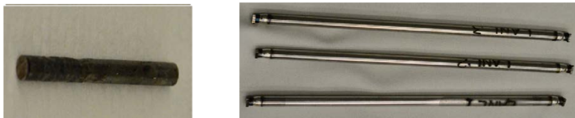
Figure 11: U-10Zr- 5% RE slug (left) and Rodlets containing metallic fuel slugs (right).
