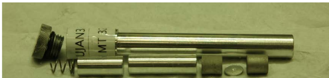
Figure 17: Rodlet 3 loading assembly configuration. From left to right; threaded cap, spring, two aluminum spacers, pellet, aluminum spacer and pellet.
