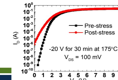
Developed an easy to use method that can be used by circuit designers to evaluate the reliability of commercial SiC MOSFETs.
