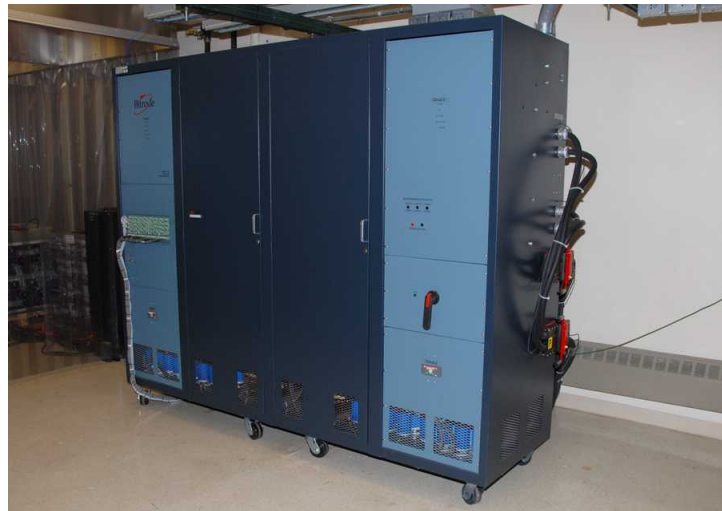
72V 1000A Bitrode (2 Channels)
