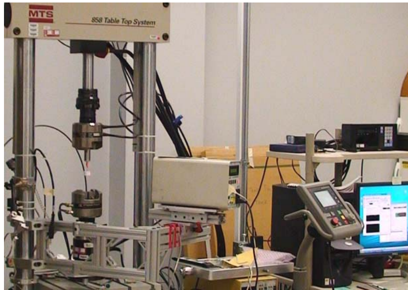
Figure 25 Torsion experimental setup of small diameter specimen.
