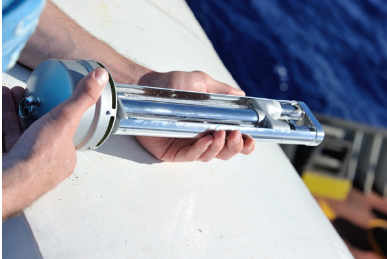
Figure 1. Assmann psychrometer, Model 430101, used in the MAGIC field campaign.
