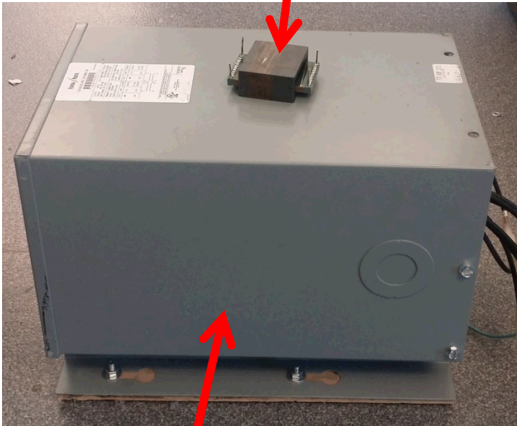
60 Hz Si-Steel Transformer 7.5 kVA – 150 lbs
