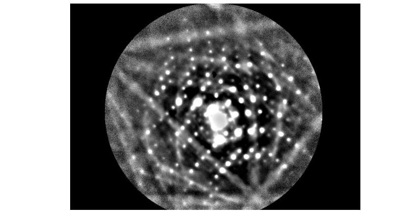
FCC pattern acquired from a very thin region of the sample with the horizontal on-axis phosphor.
