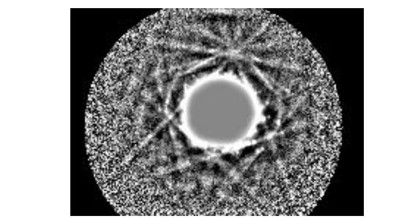
FCC pattern acquired with horizontal on-axis phosphor.
