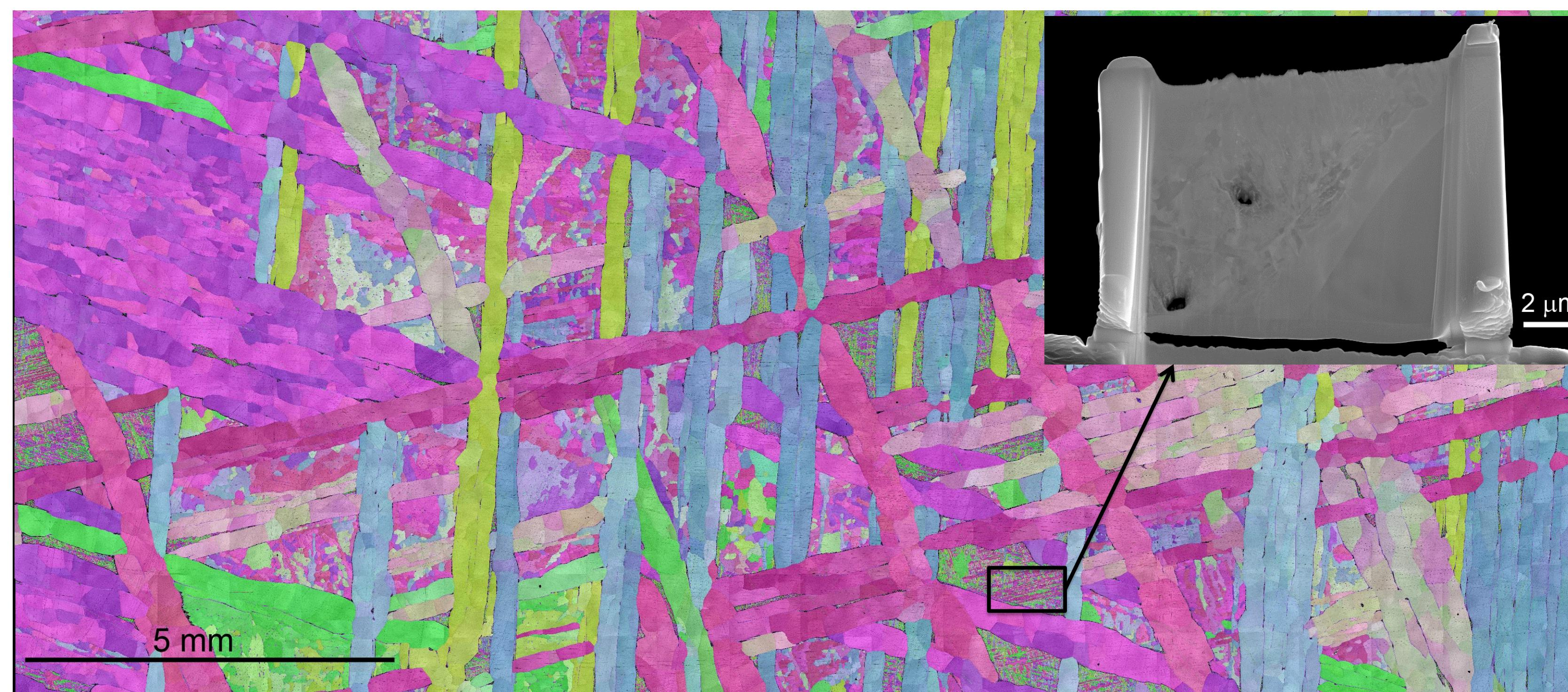
Large area orientation map of Gibeon iron meteorite prepared by standard metallographic techniques. Plessite is the fine grained areas that contain both austenite and ferrite. Inset image is of the FIB prepared thin sample milled from a region of Plessite.
