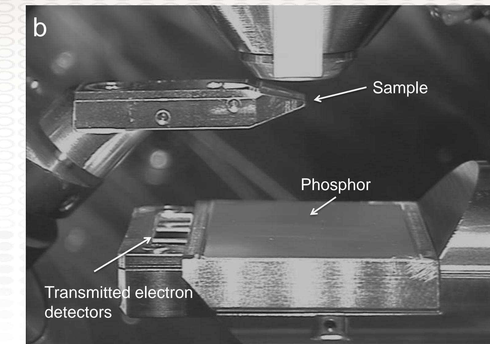
TKD has been successfully carried out on standard EBSD cameras. This geometry results in extreme pattern distortions due to the gnomonic projection. A horizontal on-axis camera arrangement (Bruker, Optimus) has been tested that removes the pattern distortion and allows lower beam currents to be used.
