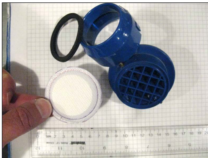
Figure 5. The LANCS bag filter was trimmed to 2.125 in (54 mm) diameter for the FAS testing.
