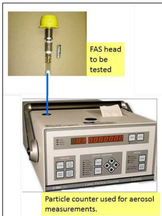
Figure 7. For the 0.3 \mu\text{m} size channel with ambient aerosol, an optical particle counter measured an 86% bypass leakage with one O-ring in the FAS holder, and 1 \times 10^{-3}\% leakage with two O-rings.
