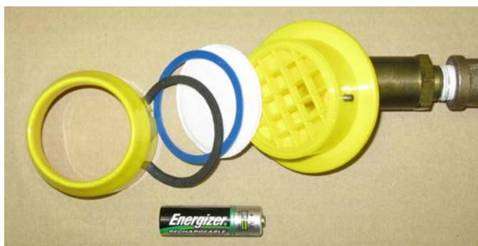
Figure 4. The LANL FAS (Fixed Air Sampler) filter holder.
