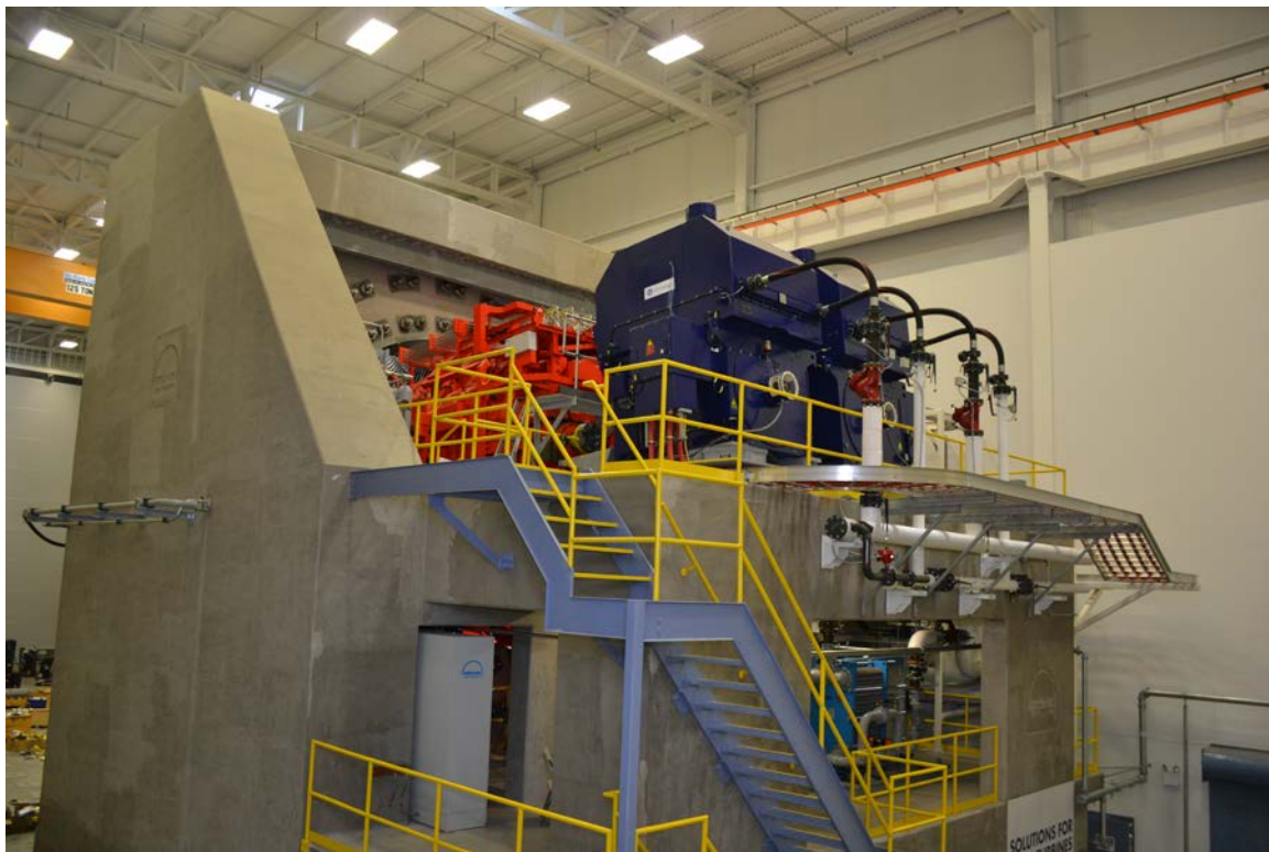
Figure 18 Rear Side of 15 MW test Rig
