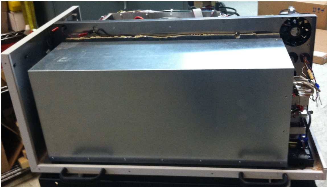
Figure 6 Fuel Cell Module Compartment of 250 Watt Generator
