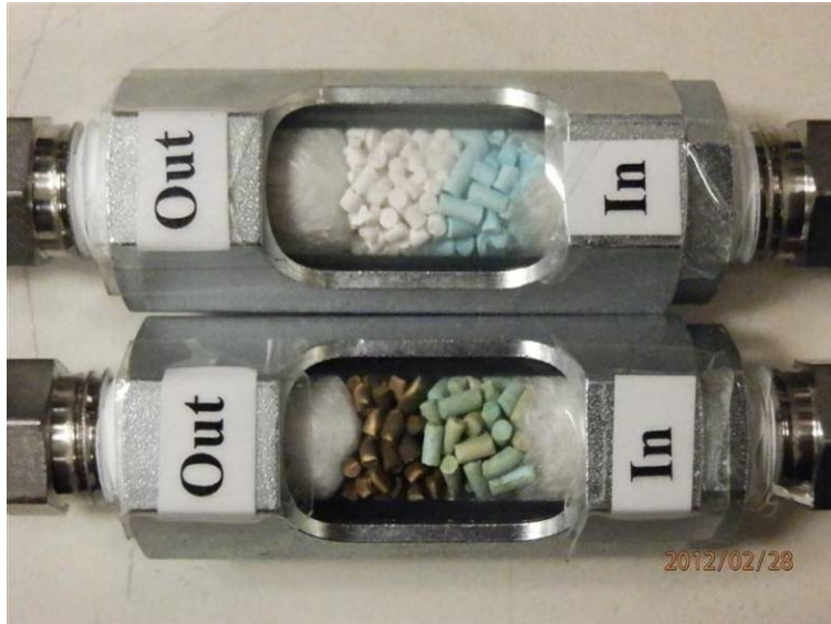
Figure 4: SulfaTrack™ showing a color change on exposure to COS
