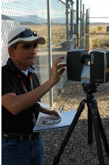
Figure 5: Scanning the Robot Vehicle Range with FARO scanner.
