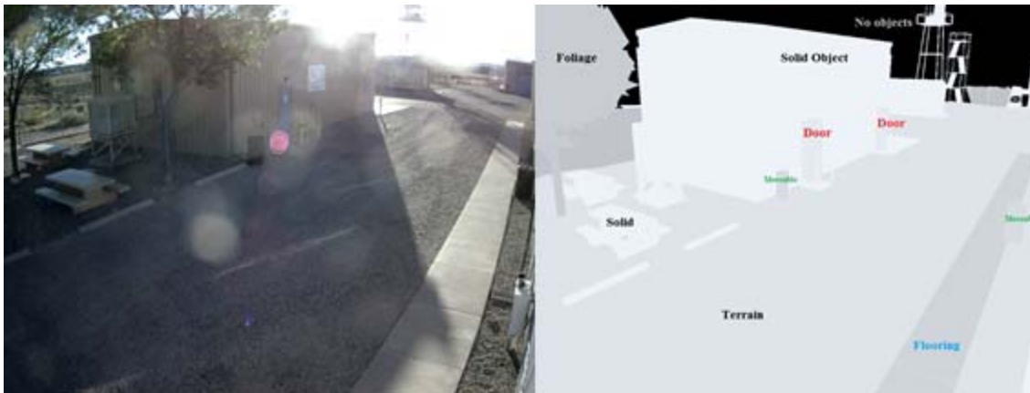
Figure 23: Using a 3D site model to systematically classify site features.
