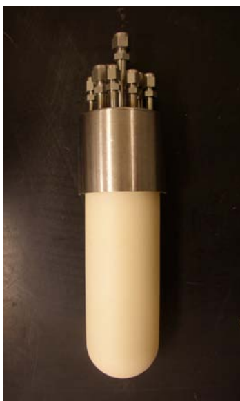
Figure 4.4 Alumina reactor for higher temperature experiments ( >1000^{\circ}\text{C} ). Tube diameter is \sim 2 \frac{3}{8} ".
