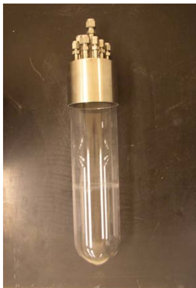
Figure 4.3 Quartz reactor for lower temperature experiments. Tube diameter is 2.25".
