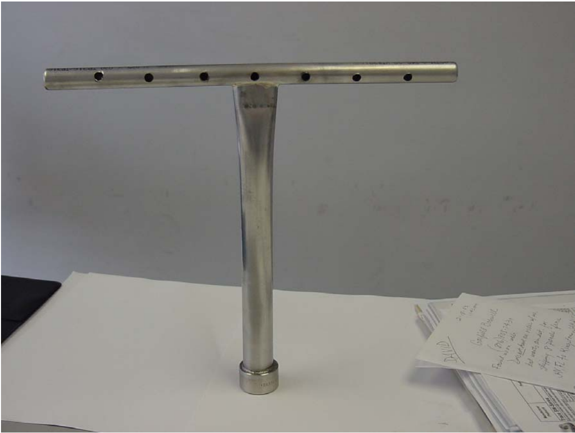
Figure E-5. RITH 6 stainless steel diffuser.
