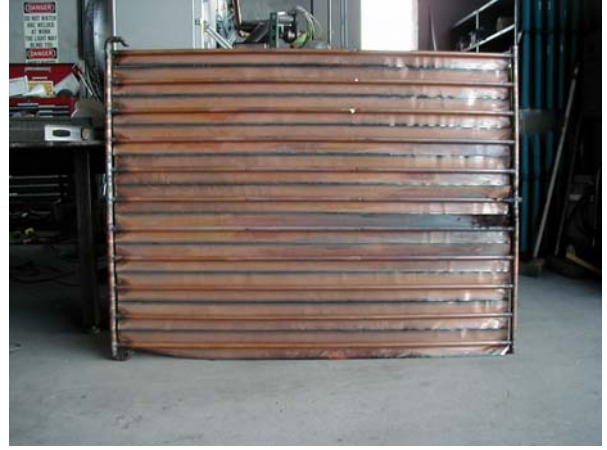
Figure 3. Backside of absorber, right side is outlet header.
