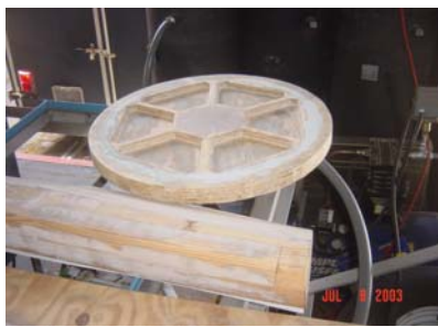
Figure 9. Wood patterns for vacuum-formed parts.
