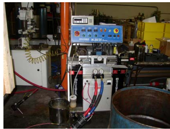
Figure 6. Gusmer foam generator.
