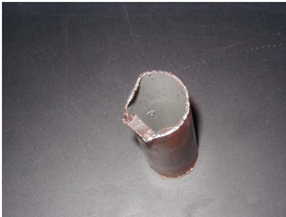
Figure 4. Sample 1A – showing inside of copper inlet header.
