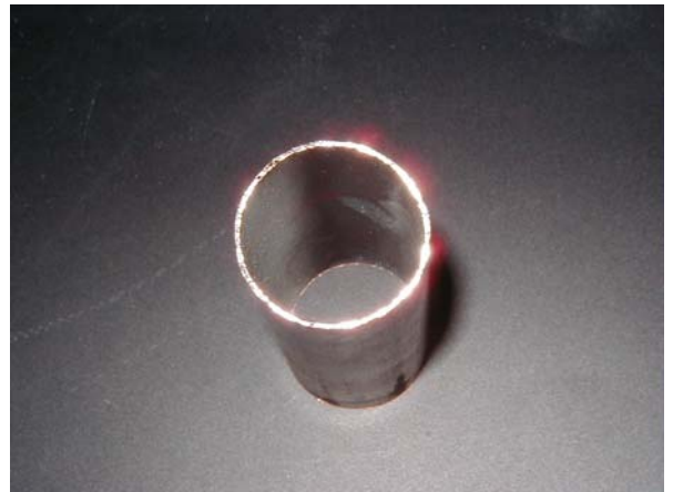
Figure 5. Sample 1B – showing inside of copper outlet header.
