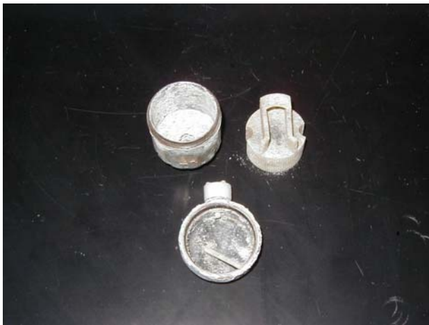
Figure 12. The inside of the vent valve. Notice the broken rod that caused the valve to leak.
