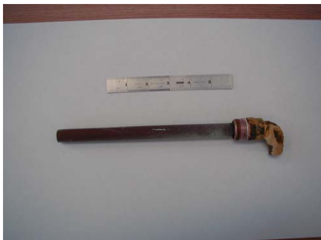
Figure 14. Another view of the inlet into the tank from the solar absorber.
