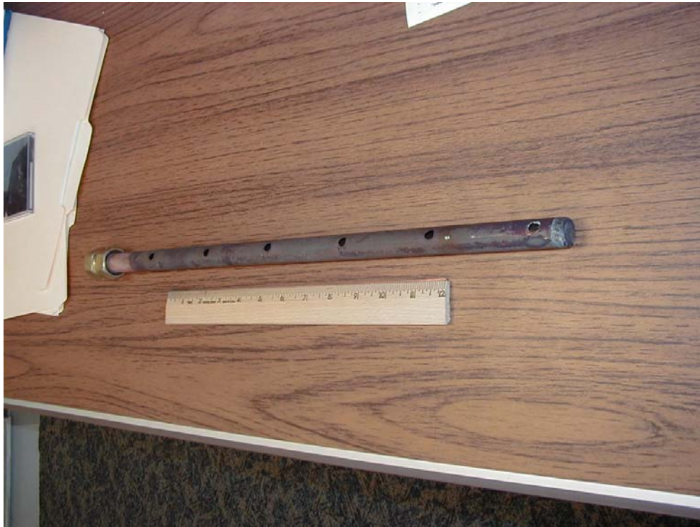
Figure E-1. Early RITH diffuser used in RITH 80 system.
