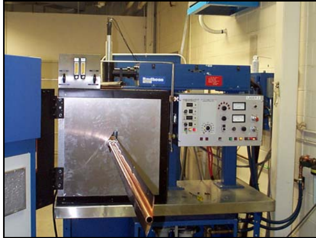
Figure 9. Riser tube and fin fed into the welder.
