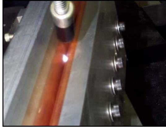
Figure 7. Laser welding of copper fin to riser tube.
