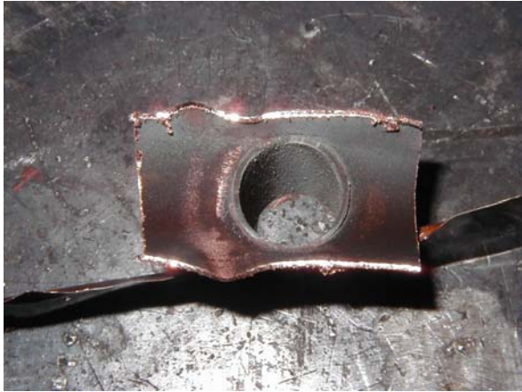
Figure 8. Sample 2C – looking down riser with cross section of the header still attached.
