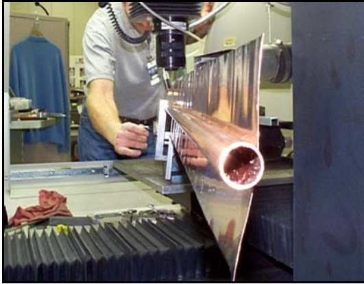
Figure 6. Test setup for welding fin to tube.
