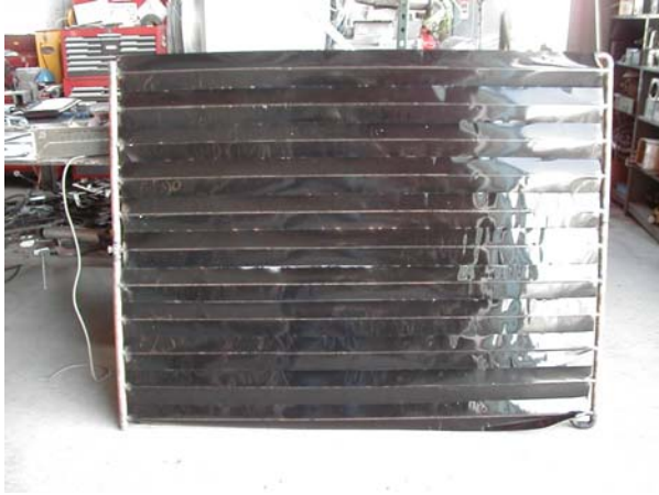
Figure 2. Front of absorber, left side is the outlet header.
