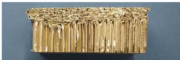
Figure 5-1. Half-crushed honeycomb specimen from Alcore.
