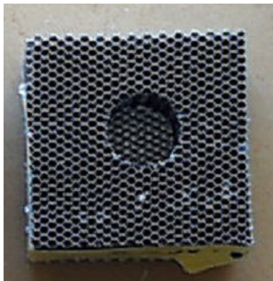
Figure 2-14. A post-experiment punch specimen of Hexcel CR-8-LC-1/8-5052-006 (22pcf).
