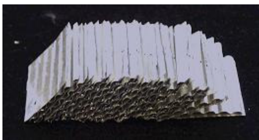
Figure 5-2. A honeycomb specimen with adhesive bond removed.
