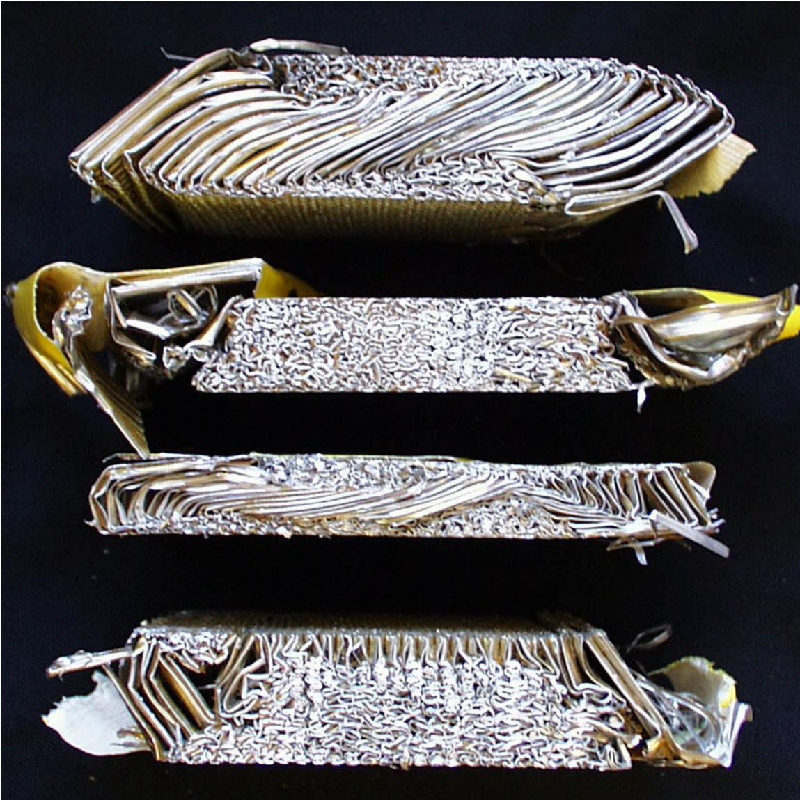
Figure 2-8. Post-experiment specimens, from top to bottom, h22t_1, h22t_2, h22t_3, and h22t_4. All were compressed in the T direction.
