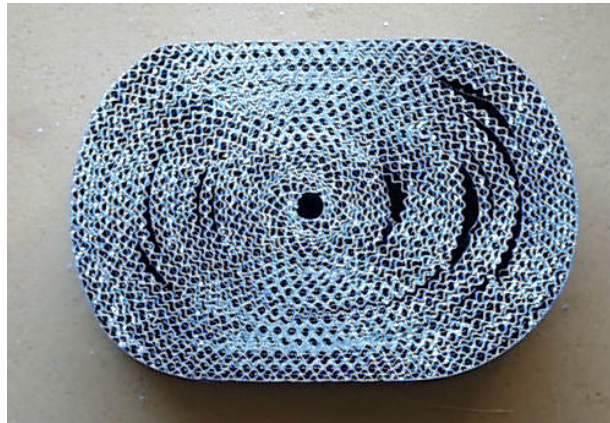
Figure 2-23. Post-experiment tube core punch specimens: 8 in. (right left) and 13 in. (left).
