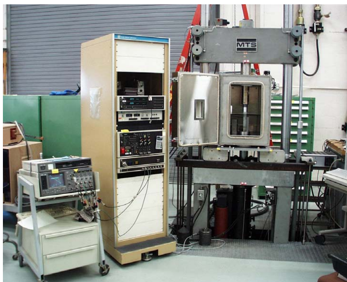
Figure 1 Experimental setup. An environmental chamber is bolted on the testing frame.
