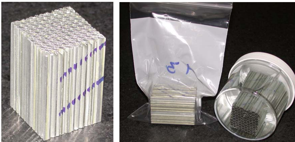
Figure 9-1. Representative specimens for the humidity effect experiment showing a dry specimen stored in bag and a wet specimen soaked in water.
