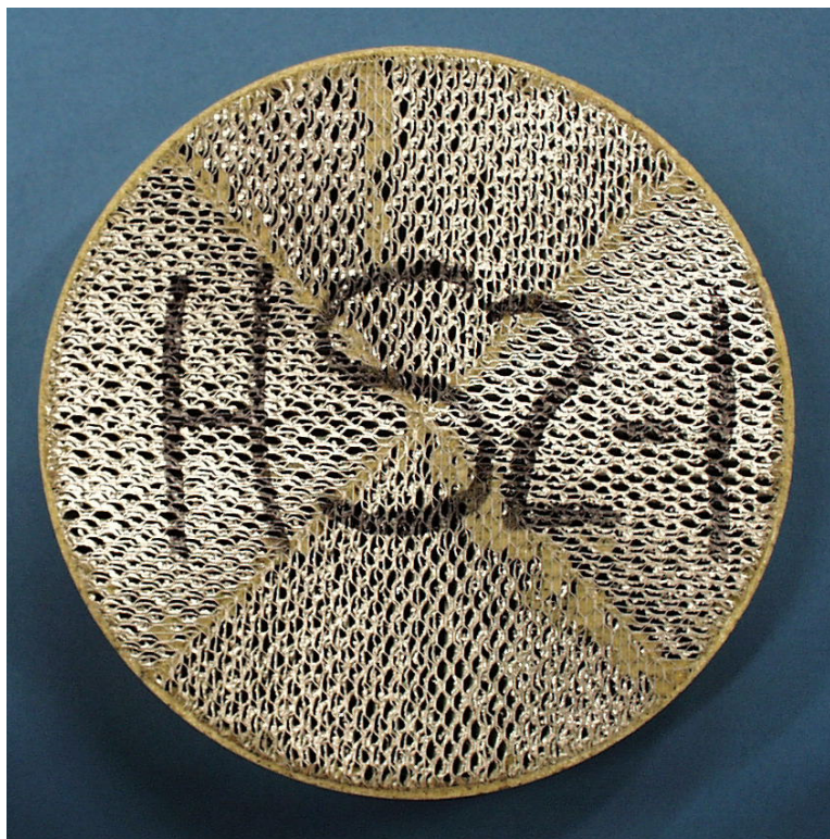
Figure 2. Sample HS2-1 before deformation. Four segments fit perfectly.
