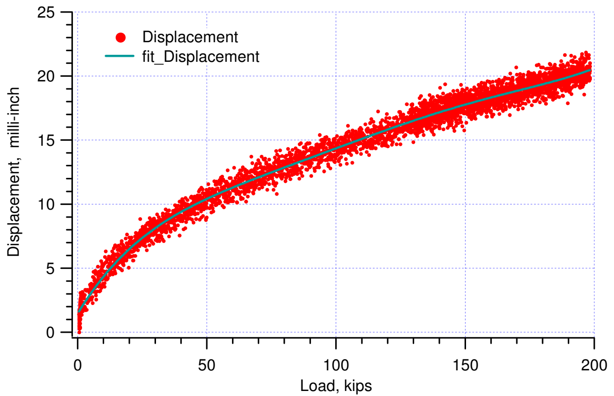
Figure 4. Compliance curve of the loading system.
