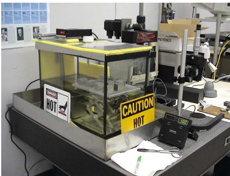
Figure 9-3. Honeycomb specimens at 70 °C and 100 percent RH.
