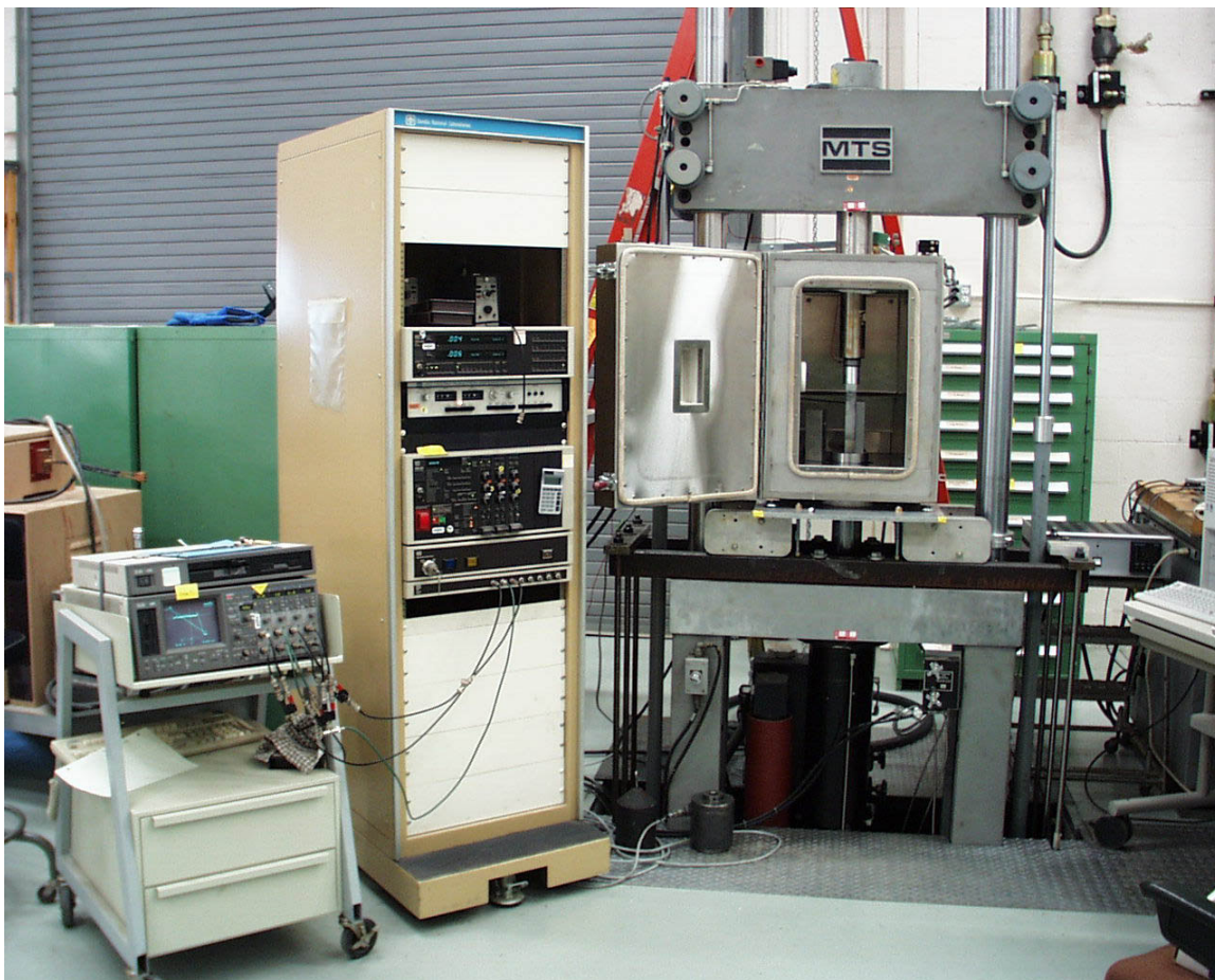
Figure 4-5. Confined compression on the MTS high-rate system.
