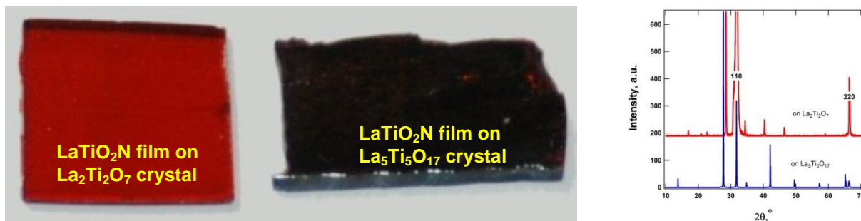
Figure 2.1a. Left: Epitaxial \text{LaTiO}_2\text{N} thin films were prepared on top of substrates of transparent single crystals of insulating \text{La}_2\text{Ti}_2\text{O}_7 and on black single crystals of conductive \text{La}_5\text{Ti}_5\text{O}_{17} . Right: Diffraction patterns show the crystallographic co-alignment of perovskite \text{LaTiO}_2\text{N} film peaks (110 and 220 when indexed to an idealized cubic cell) with the corresponding perovskite-like peaks of the more complex layered perovskite structure of substrates.
